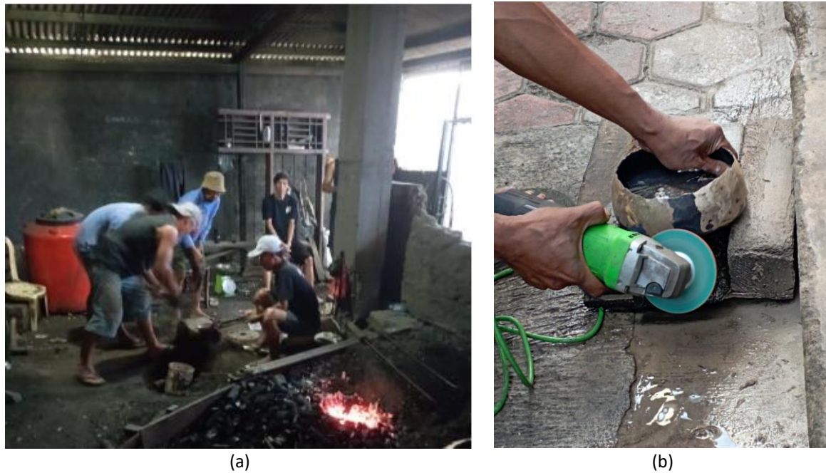
Fig. 3. Forging Stage (a) Forging by gamelan craftsmen (b) Smoothing the forged gamelan with a grinding machine
