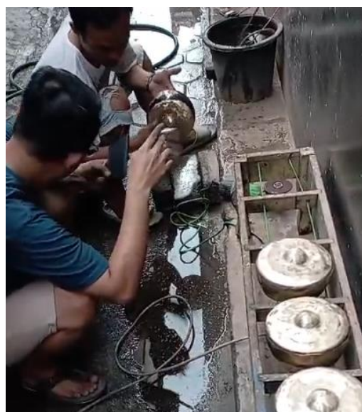
Fig. 4. Tone tuning stage with the help of tones already stored on the smartphone
