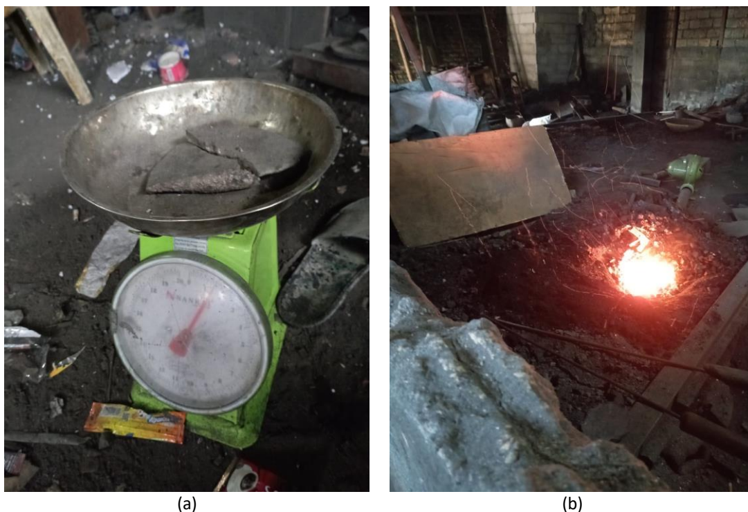
Fig. 1. Melting Stage (a) scales for measuring metal mixtures to be smelted (b) preparations for melting metal mixtures
