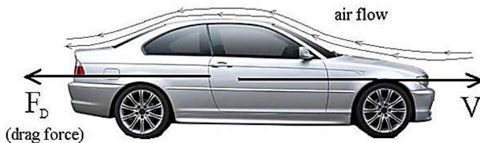
Fig. 1. Drag force on a car [14]
