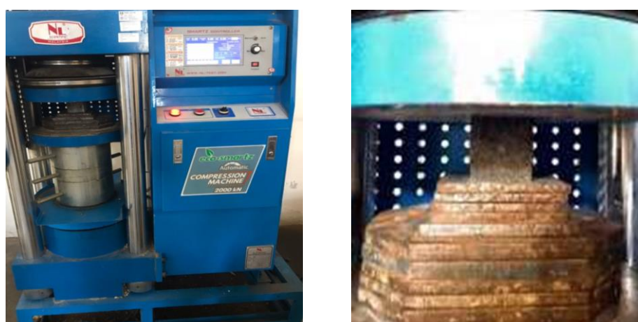
Fig. 5. Mortar testing on compressive strength test equipment
