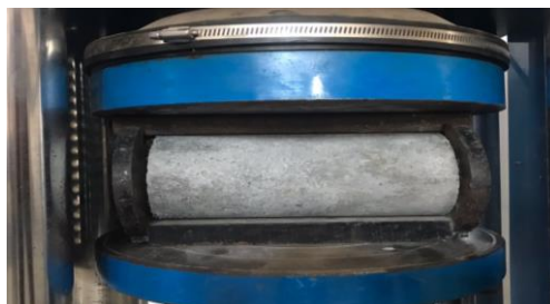
Fig. 6. The splitting tensile test setup
