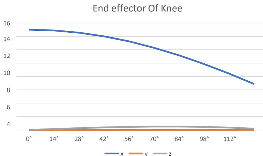
**Fig. 12.** Graph illustrating the position of the Knee end effector during the heel slide exercise
