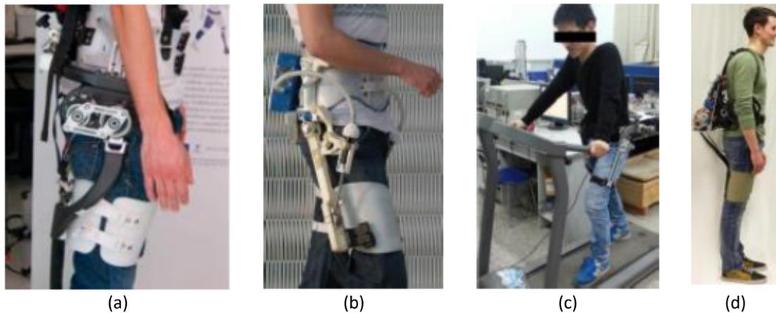
**Fig. 1.** (a) Exoskeleton Developed by Giovacchini *et al.*, [13], (b) Hipso (Hip Ball Screw Orthosis) [14], (c) PH-EXOS [15], (d) Exosuit [16]
