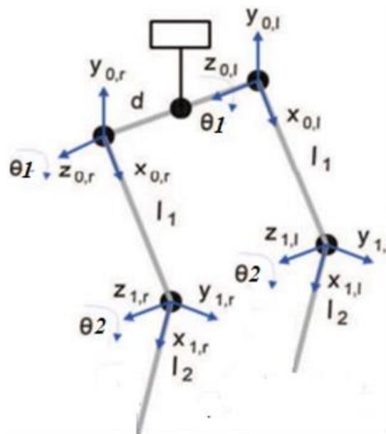
**Fig. 3.** Distribution of Reference Planes on the Exoskeleton of the lower limb [22]
