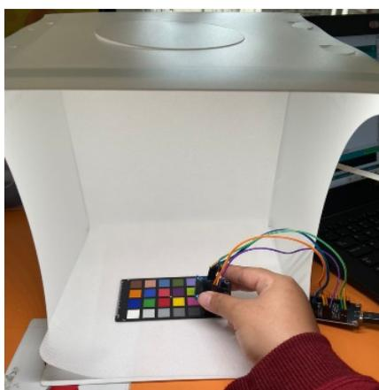
**Fig. 3.** Color measurement in Puluz photo light box
