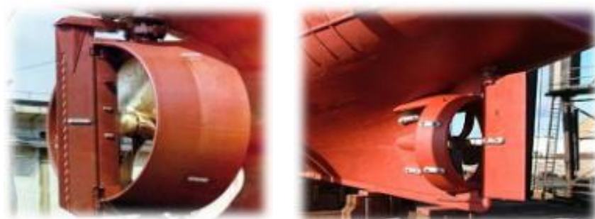
Fig. 2. Tipe kort nozzle, (left) Rotation nozzle view and (right) Fixed nozzle view [9]
