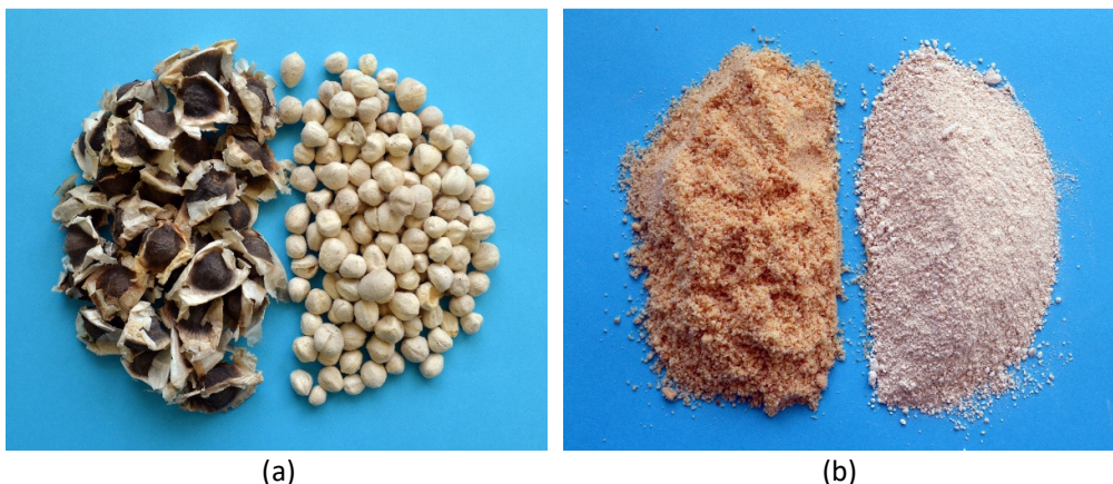
Fig. 1. (a) Unshelled and shelled MO seeds, (b) crude seeds powder (light brown color) and defatted seeds powder (white color)
