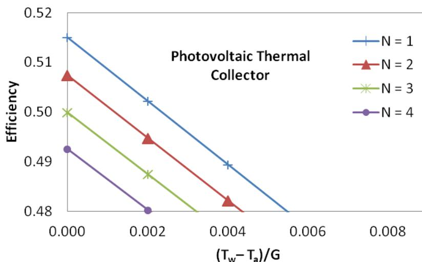
**Fig. 2.** Corrected Characteristics for Photovoltaic Thermal Collector Based on Number of Modules at Constant Flow Rate ( $\dot{m} = 0.122$  kg/s)
