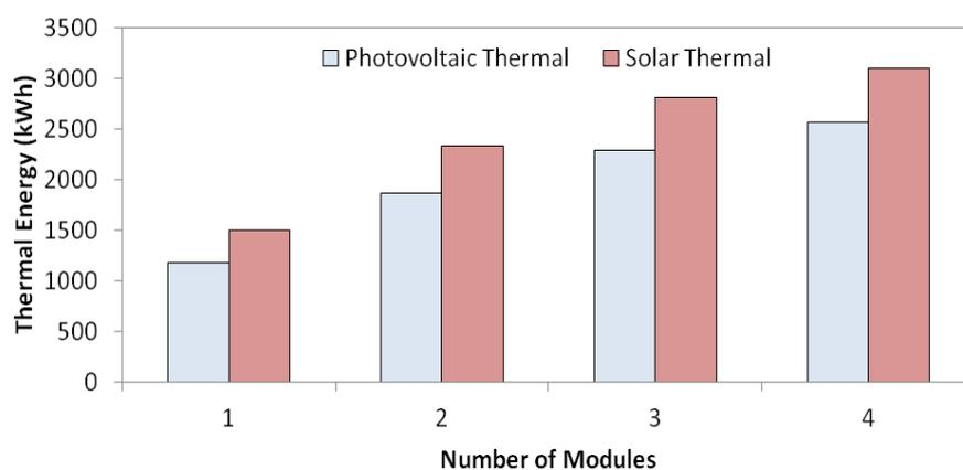
**Fig. 6.** Comparative Result of Thermal Heating Energy Generated by System Based on Number of Modules at Constant Flow Rate ( $\dot{m} = 0.122 \text{ kg/s}$ )
