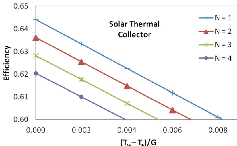
**Fig. 3.** Corrected Characteristics for Solar Thermal Collector Based on Number of Modules at Constant Flow Rate ( $\dot{m} = 0.122$  kg/s)
