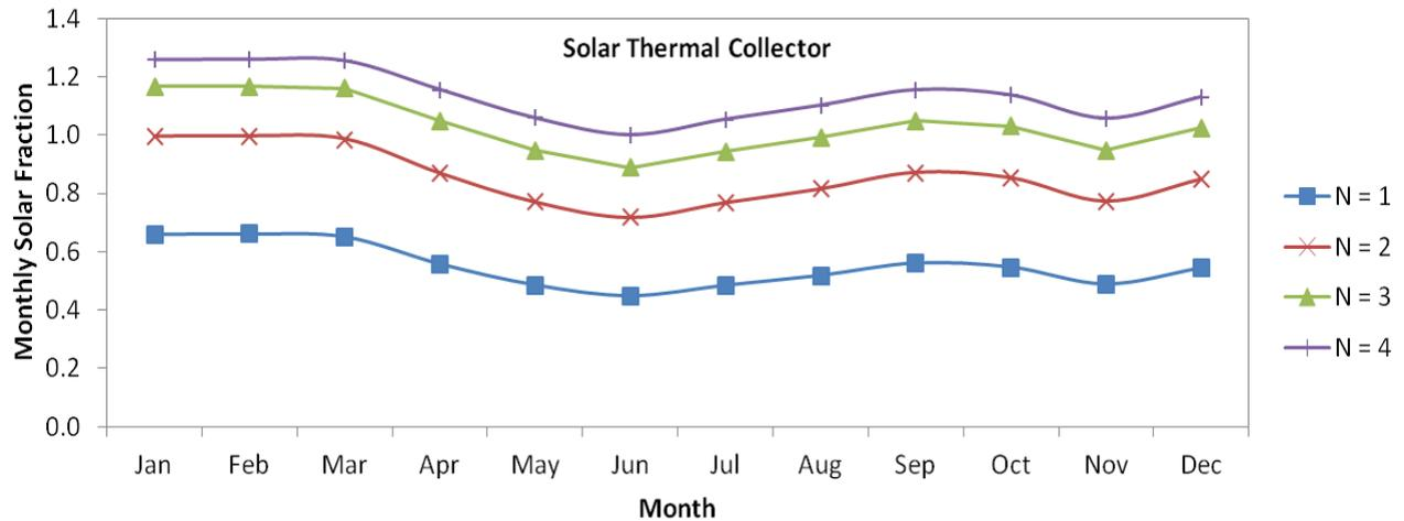
**Fig. 5.** Result of Solar Thermal Water Heating System Based on Number of Modules at Constant Flow Rate ( $\dot{m} = 0.122 \text{ kg/s}$ )
