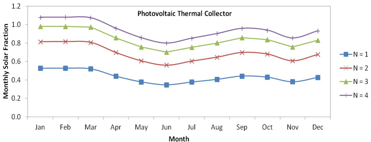
**Fig. 4.** Result of Photovoltaic Thermal Water Heating System Based on Number of Modules at Constant Flow Rate ( $\dot{m} = 0.122 \text{ kg/s}$ )
