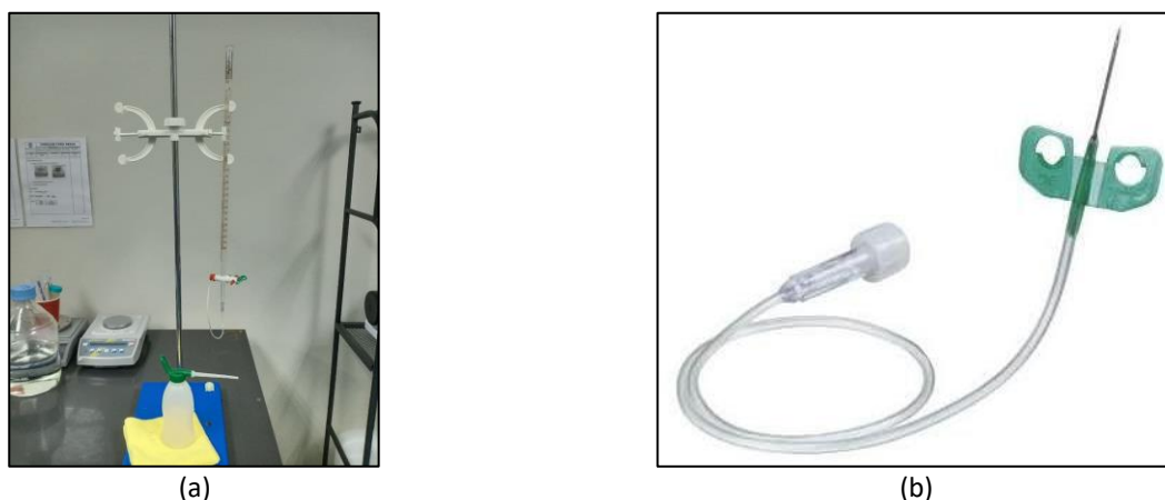
Fig. 4. (a) Burette setup with Butterfly-needle 21G hold on retort stand (b) Butterfly needle 21G with connector [Note: Burette setup for draw volume test for experiment 1 and experiment 2 (test2)]
