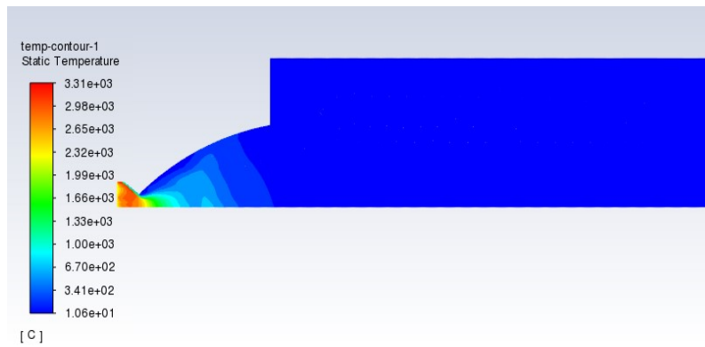
Fig. 9. Static temperature of Mach 2
