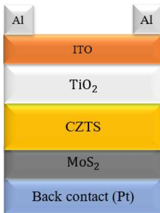
Fig. 1. The structure of the proposed device
