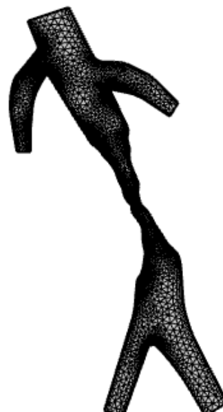
Fig. 4. Free-triangular moving mesh of the stenosed artery (11,153 elements)
