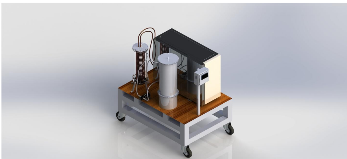
Fig. 2. Three-dimensional design components ethanol refinery condenser in cooking oil production mini plant
