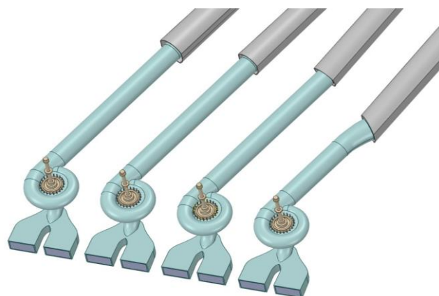
Fig. 4. Francis turbine with dual outlet model
