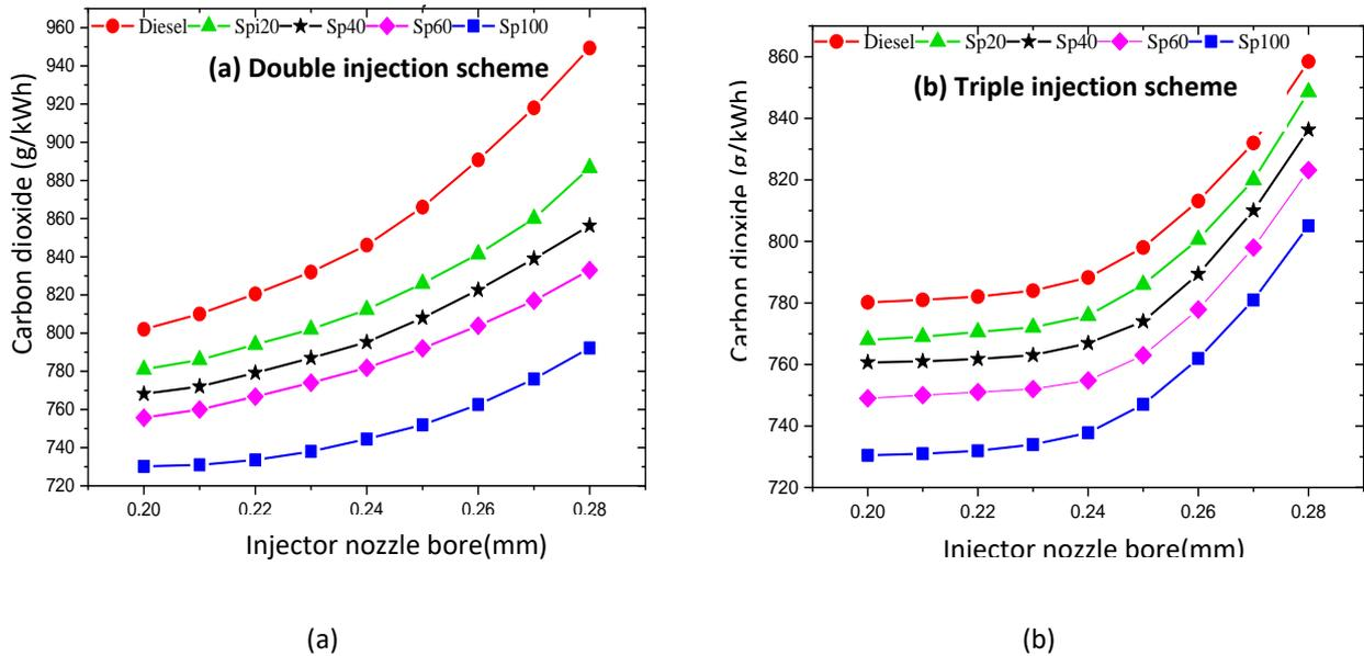
**Fig. 11.** Emission of carbon dioxide versus injector nozzle bore (a) Double injection (b) Triple injection scheme
