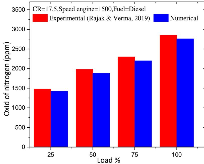
Fig. 5. NO<sub>x</sub> emission variations versus engine load
