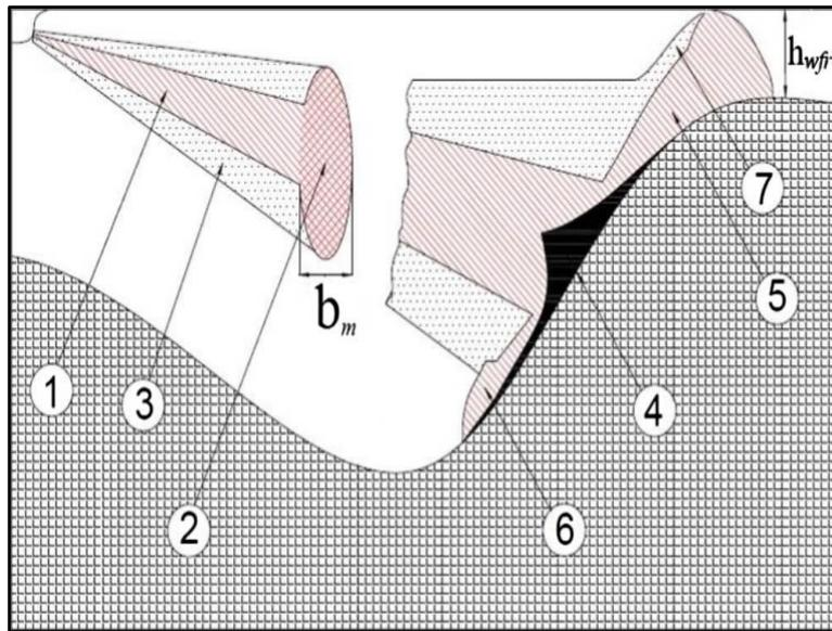
Fig. 2. Various zones of diesel spray [27]
