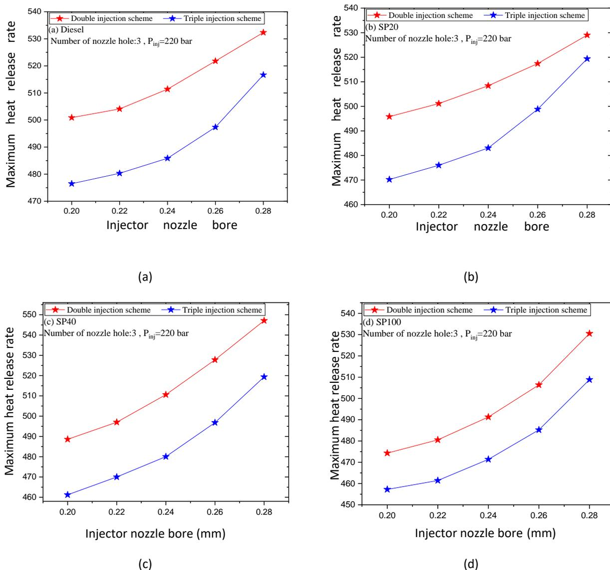
Fig. 9. Maximum heat release rate versus injector nozzle bore (a) Diesel (b) SP20 (c) SP40 (d) SP100
