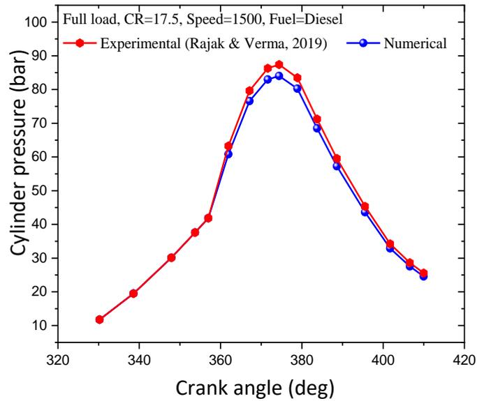
Fig. 3. Cylinder pressure variation with crank angle
