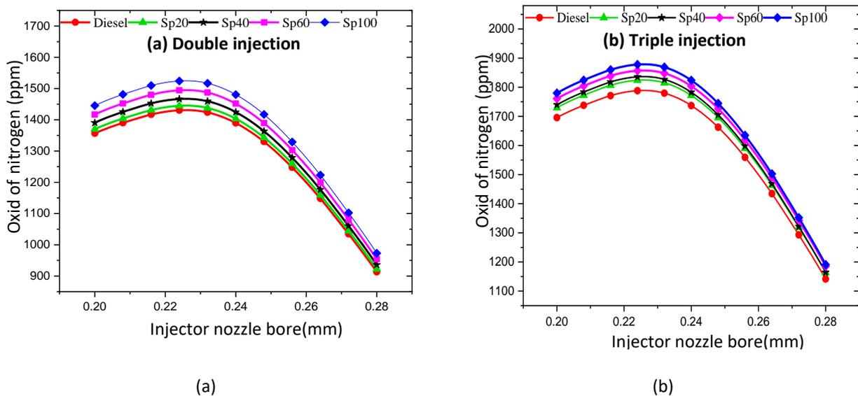
**Fig. 10.** Emission of  $\text{NO}_x$  versus injector nozzle bore (a) Double injection (b) Triple injection
