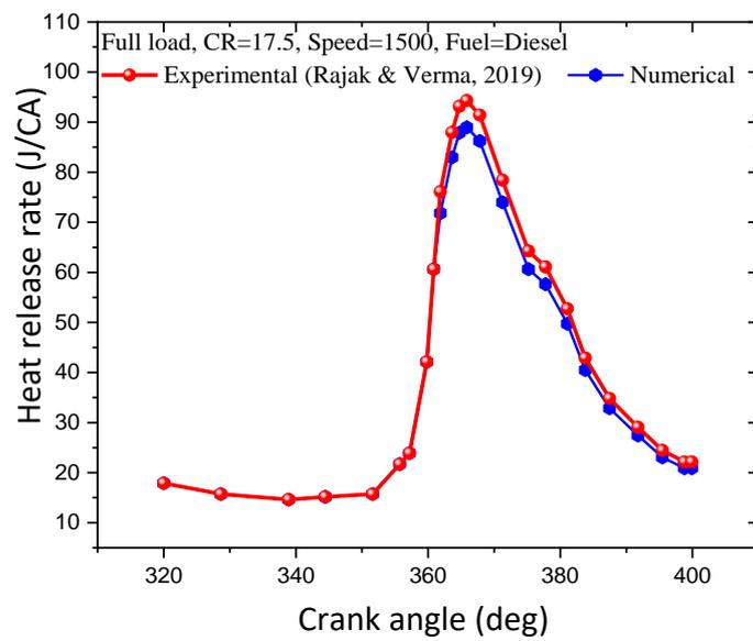
Fig. 4. Heat release rate variation versus crank angle
