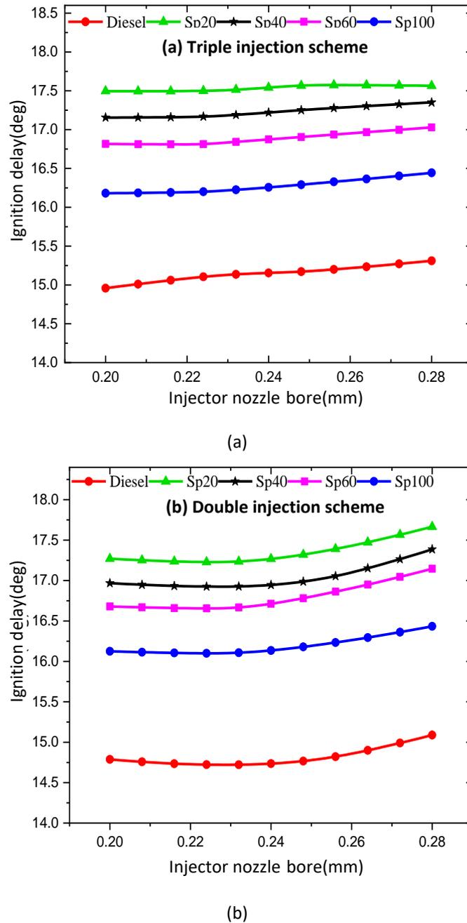
**Fig. 6.** Ignition delay versus injector nozzle bore (a) Triple injection scheme (b) Double injection scheme
