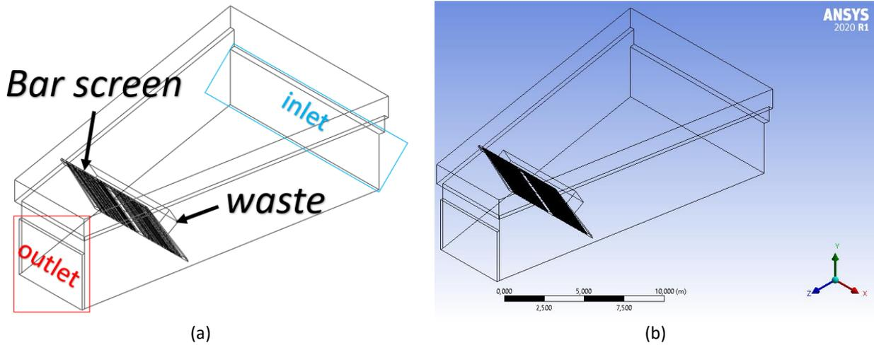
**Fig. 1.** Simulation setup (a) Determination of boundary condition (b) Visualization of boundary conditions
