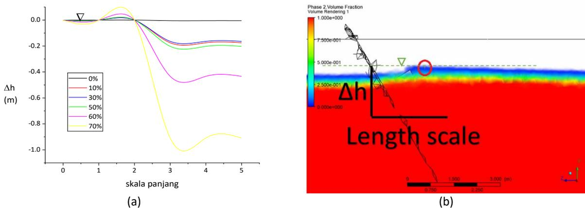
**Fig. 6.** Estimation of  $\Delta h$  for garbage 0 – 70%: (a)  $\Delta h$  prediction of CFD results; and (b) Visualization of  $\Delta h$  on the condition of the percentage of garbage 50%
