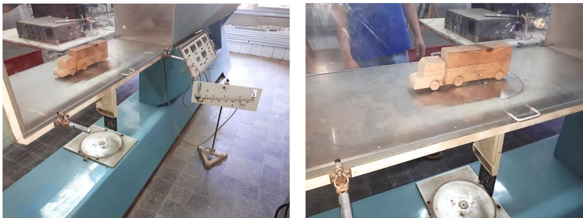
Fig. 7. Truck model inside the test section of wind tunnel of aerodynamics laboratory
