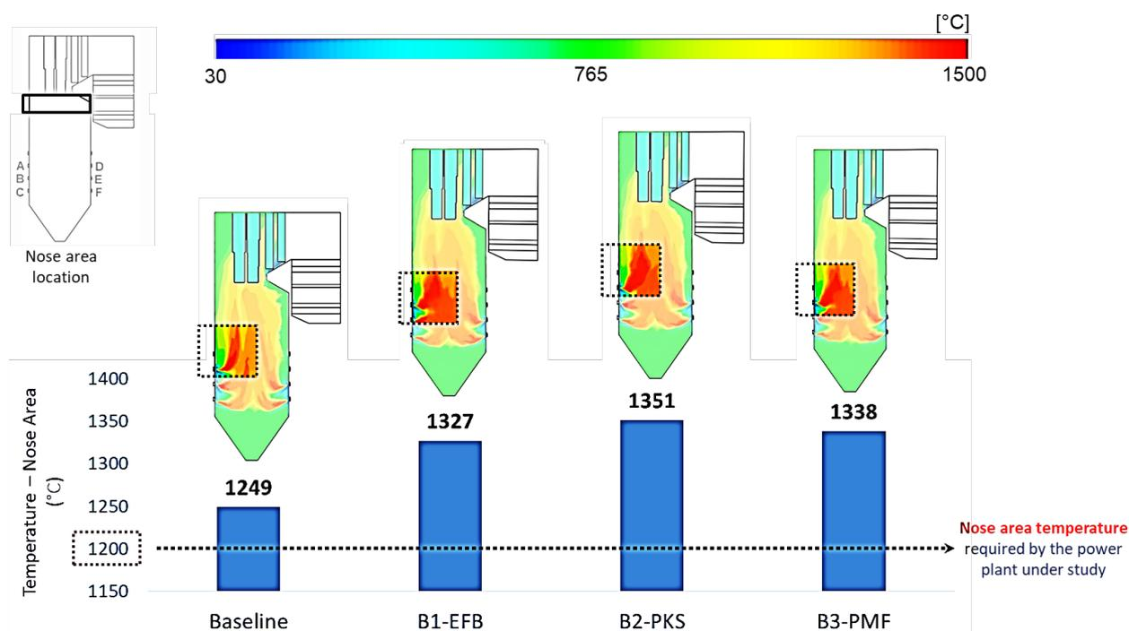
**Fig. 3.** Predicted temperature results within the boiler model
