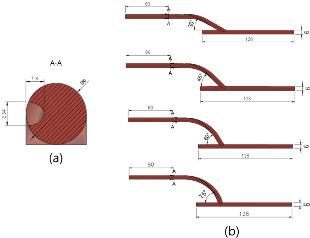
**Fig. 1.** (a) Cross-sectional profile of the graft in sections A-A; (b) Models with varying anastomosis angles
