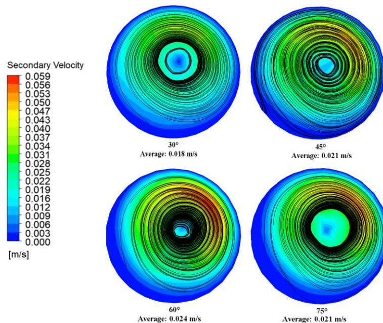
**Fig. 5.** Secondary velocity contours and crossflow streamlines according to anastomosis angle. (a) 30°; (b) 45°; (c) 60°; (d) 75°
