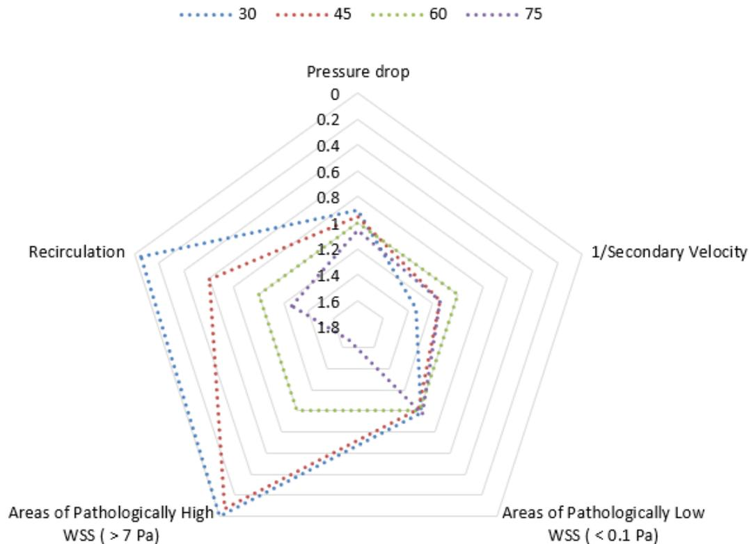
**Fig. 6.** Comparison of pressure drop, secondary velocity, areas of pathologically low and high WSS, and recirculation across different anastomosis angles
