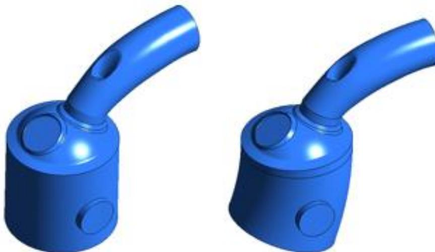
Fig. 2. Model of (left) Straight Cylinder Liner and (right) Curve Cylinder Liner
