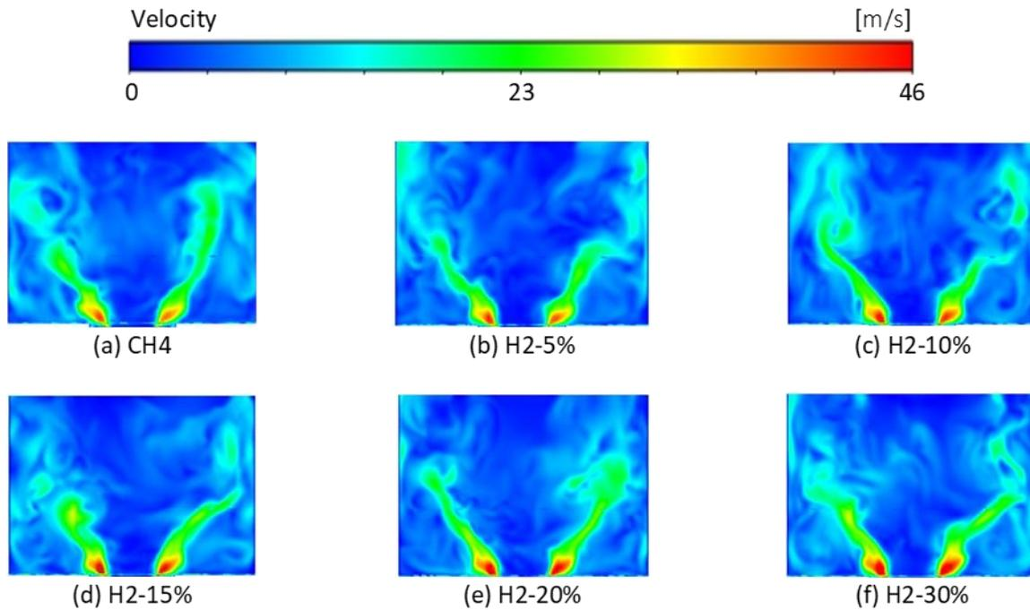
Fig. 5. Predicted velocity magnitude contours
