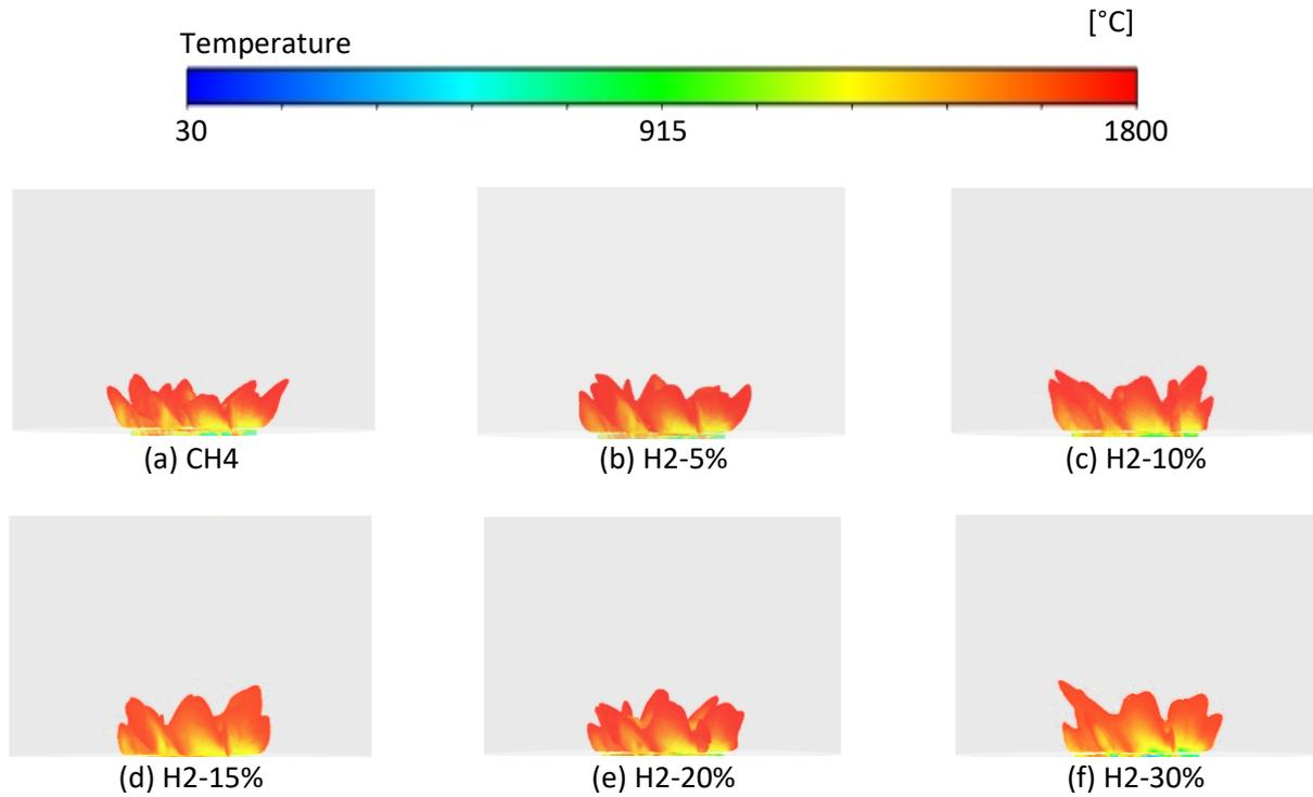
Fig. 7. Predicted flame front contours
