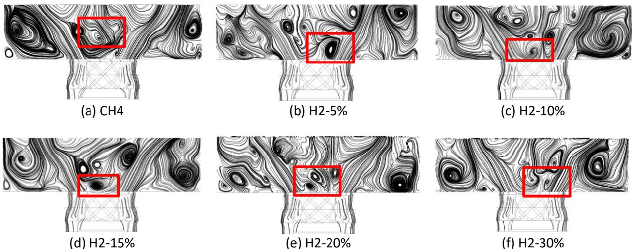
Fig. 8. Predicted flow streamlines
