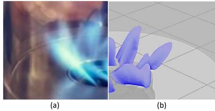
**Fig. 3.** Flame fronts between the (a) actual experiment and (b) numerical studies
