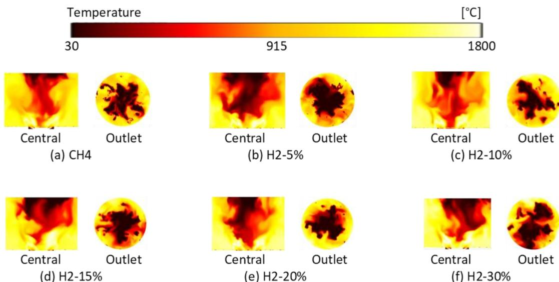
**Fig. 4.** Predicted temperature contours
