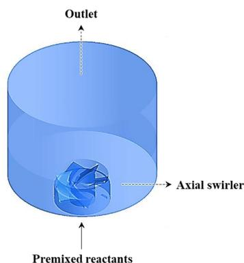
**Fig. 1.** Computational domain of the swirl burner
