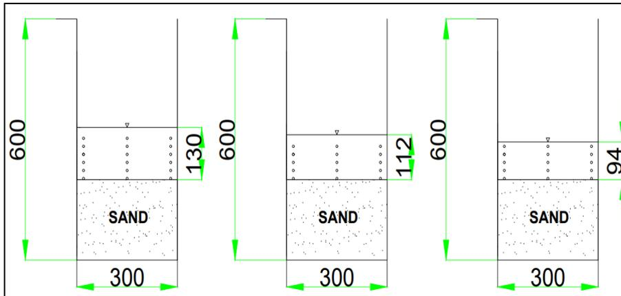
Fig. 4. Cross-section of water sampling points for each station along the meandering channel with different freshwater discharge and water depth
