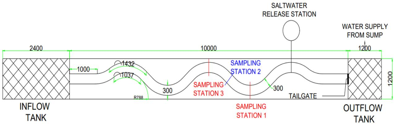
Fig. 1. Diagram of the meandering channel layout
