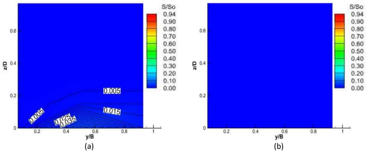
**Fig. 7.** Salinity profile of Section 1 (a) at bend apex and Section 2 (b) at cross-over. The contour represents the isohaline of water intrusion at Case 2 ( $Q_f = 4.8$  L/s)
