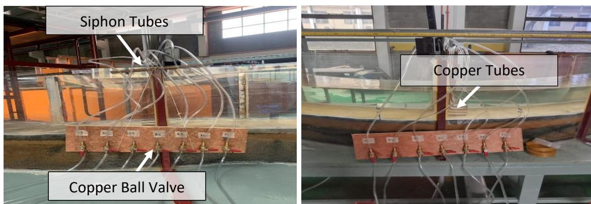
Fig. 2. A self-made siphoning device in a meandering channel
