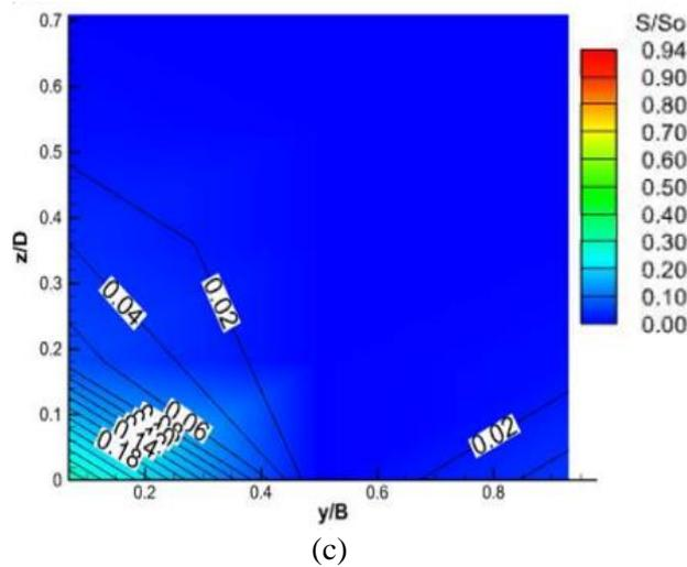
**Fig. 6.** Salinity profile of Section 1 (a) at bend apex, Section 2 (b) at cross-over and Section 3 (c) at bend apex. The contour represents the isohaline of water intrusion at Case 2 ( $Q_f = 3.2$  L/s)
