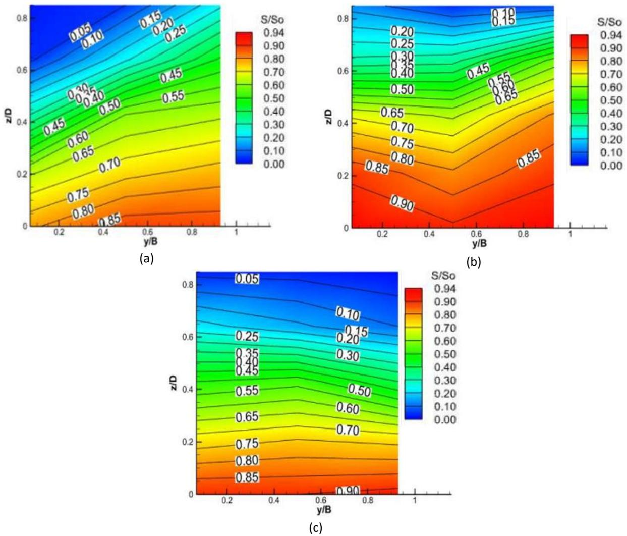
**Fig. 5.** Salinity profile of Section 1 (a) at bend apex, Section 2 (b) at cross-over and Section 3 (c) at bend apex. The contour represents the isohaline of water intrusion at Case 1  $Q_f = 2.4$  L/s
