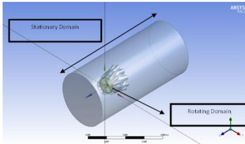
**Fig. 2.** Numerical domain on the jet-engine inspired Wind Turbine
