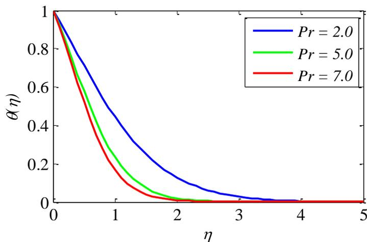
**Fig. 14.** Effect of Pr on temperature profile
