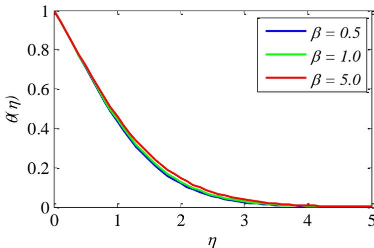
Fig. 3. Effect of  $\beta$  on temperature profile
