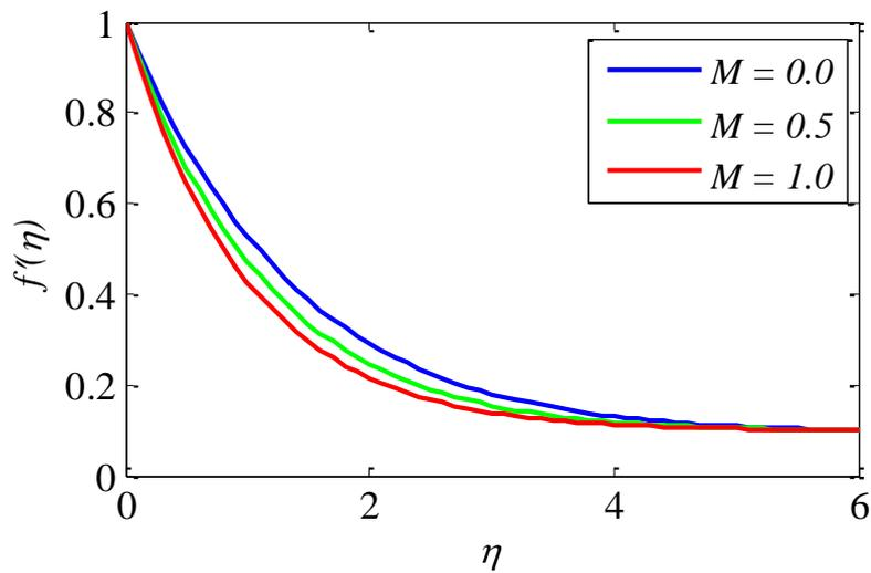
Fig. 5. Effect of  $M$  on velocity profile
