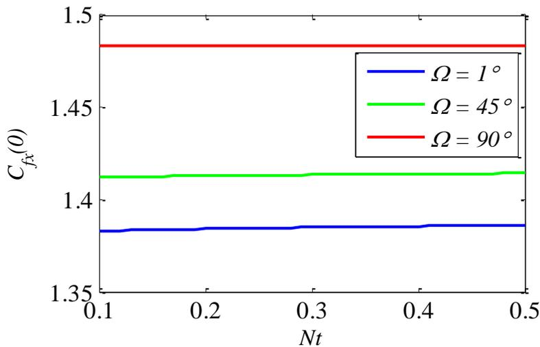
Fig. 23. Effect of  $Nt$  and  $\Omega$  on skin friction coefficient
