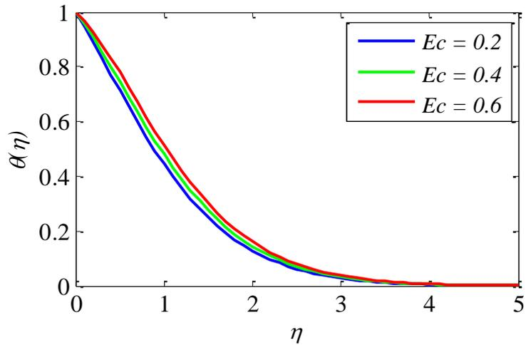
Fig. 16. Effect of  $Ec$  on temperature profile
