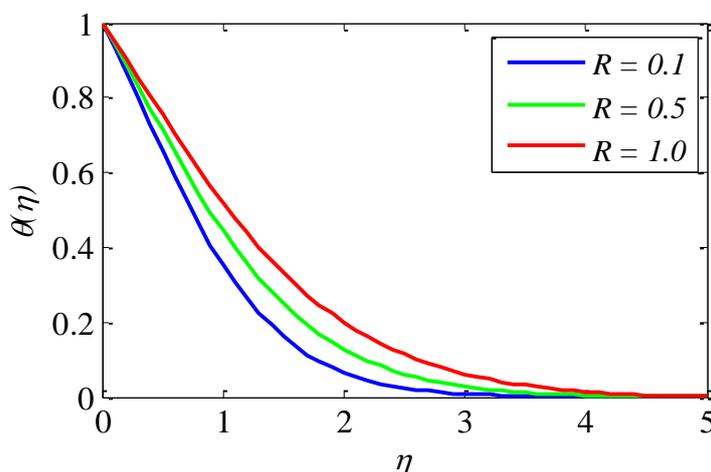
**Fig. 15.** Effect of  $R$  on temperature profile
