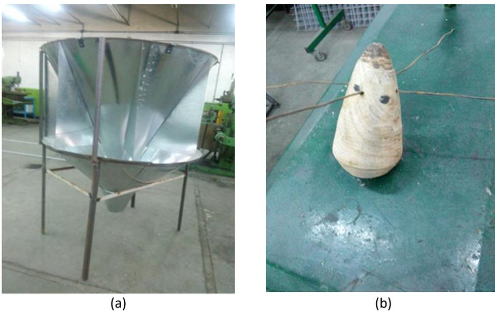
**Fig. 2.** (a) Fabricated wind channel, (b) Fabricated diffuser
