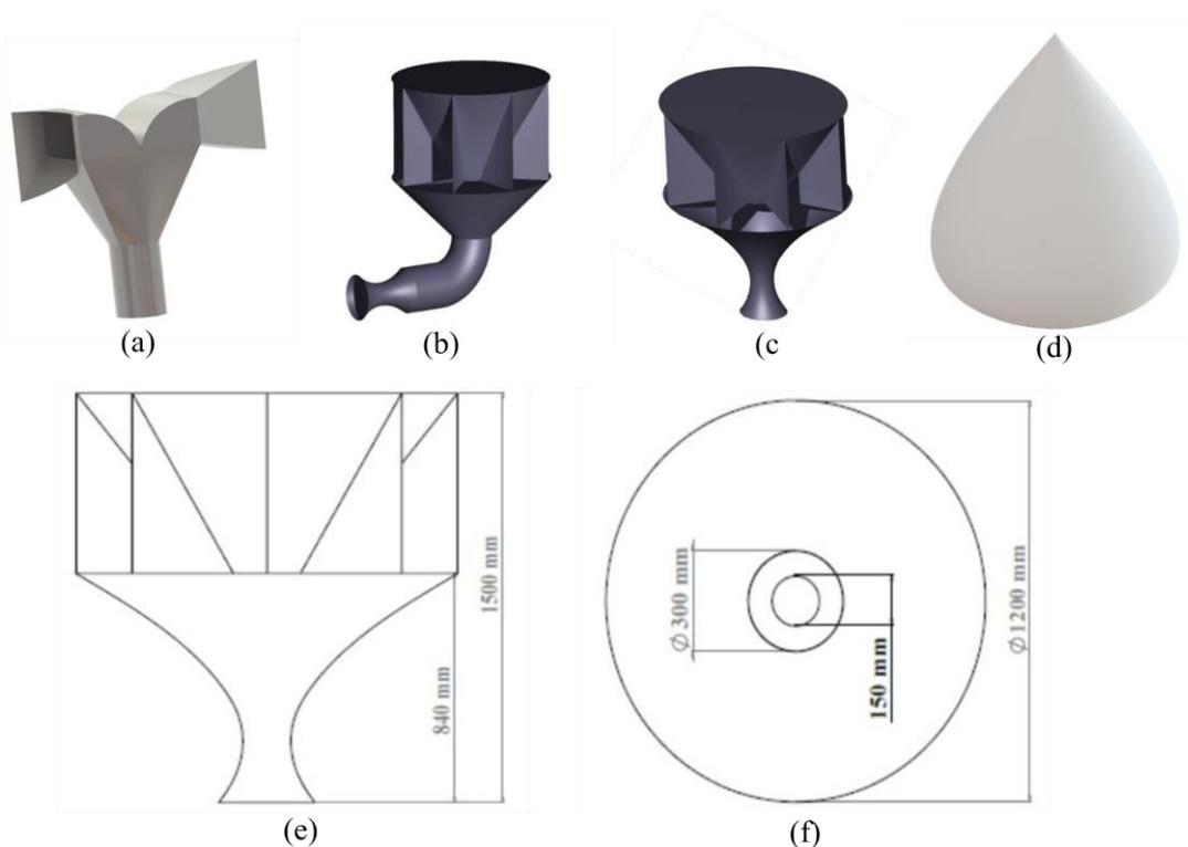
**Fig. 3.** Geometry of the created channels: (a) wind channel 1; (b) wind channel 2; (c) wind channel 3; (diffuser); (e) Accurate dimensions and wind channel 3 geometry; (f) configuration by eight 45° entries
