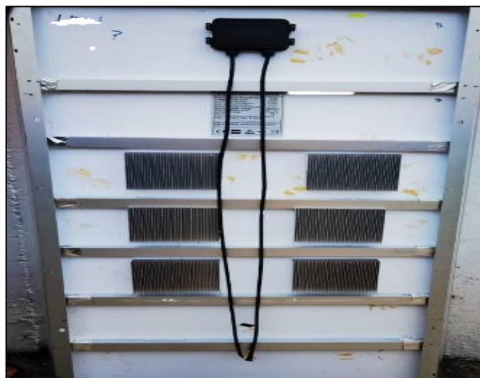
Fig. 4. Design of passive cooling system in hardware
