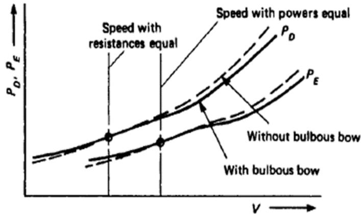
Fig. 1. Comparison of resistance between hull with and without bulbous bow [7]
