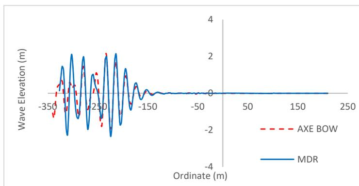
**Fig. 10.** Wave Elevation in Various Bow Shapes
