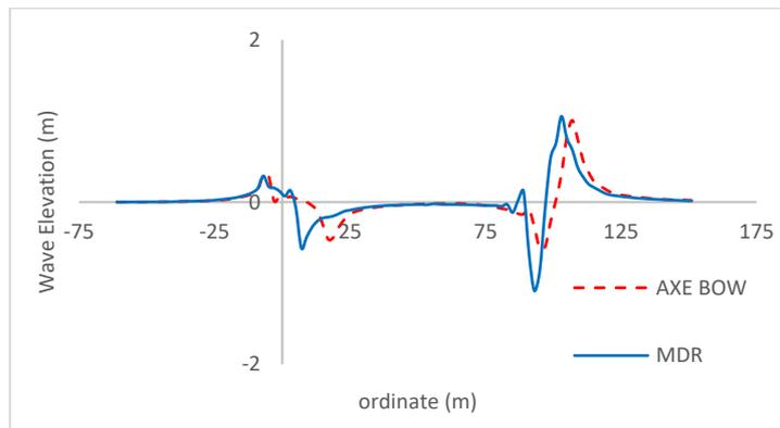
**Fig. 8.** Wave Elevation in Various Bow Shapes by CFD
