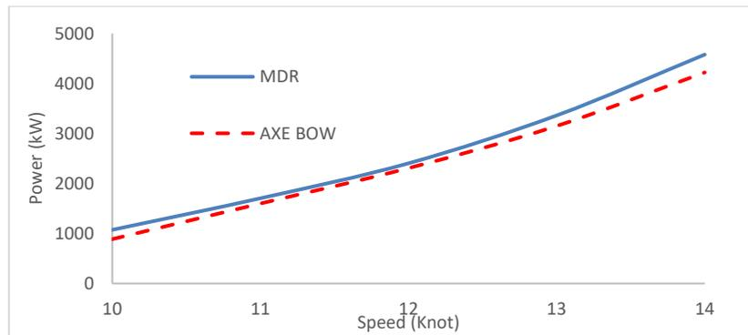
**Fig. 12.** Power v Speed Curves
