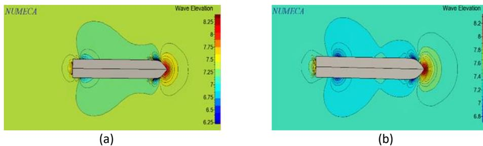
Fig. 7. Wave Elevation in Various Bow Shapes by using CFD Numeca (a) Moor Deep Ram Bow, (b) Axe Bow
