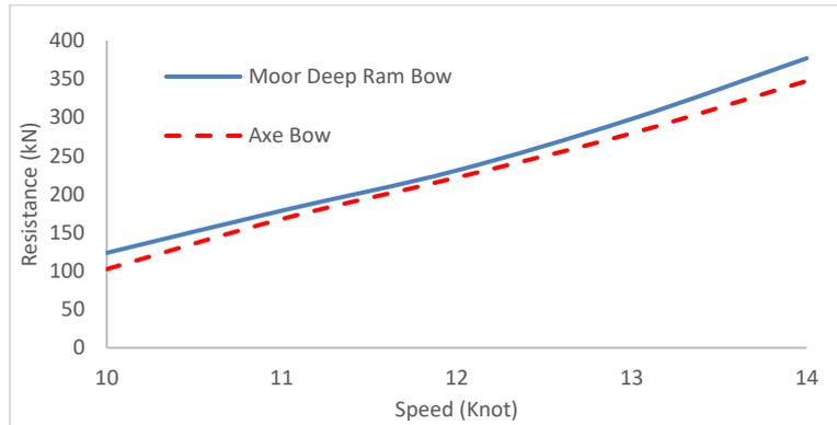
Fig. 6. Graph of resistance v speed on various bow types
