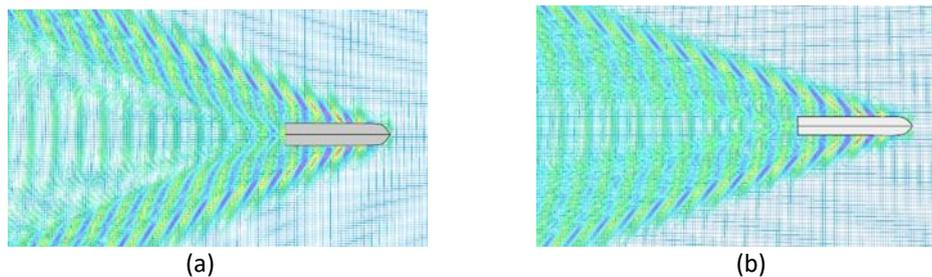
**Fig. 9.** Wave Patterns in Various Bow Shapes (a) Moor Deep Ram Bow, (b) Axe Bow
