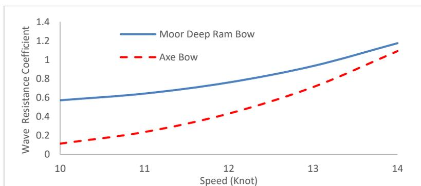
**Fig. 11.** Wave Resistance Coefficient v Speed
