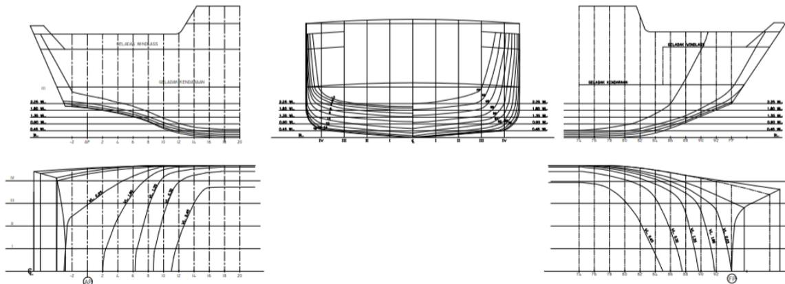
**Fig. 1.** Lines Plan of KMP. Bontoharu 1050 GT
