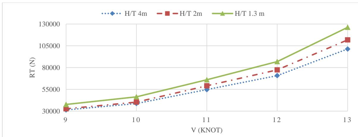
**Fig. 7.** KMP Bontoharu Ship Resistance with Depth Variation
