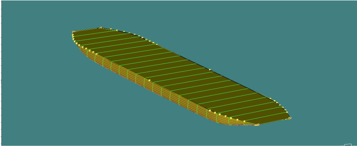
**Fig. 2.** KMP Bontoharu Hull Model on Maxsurf Modeler
