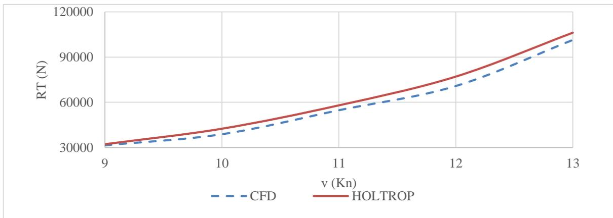
Fig. 6. Comparison of CFD Ship Resistance with Holtrop
