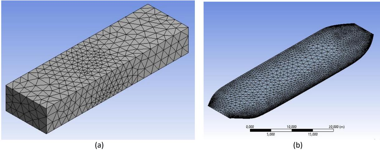
**Fig. 4.** (a) Hull Meshing (b) Meshing with Fluid Domain
