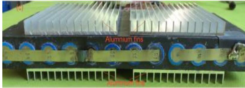
Fig. 9. Composite PCM with aluminium fins [93]
