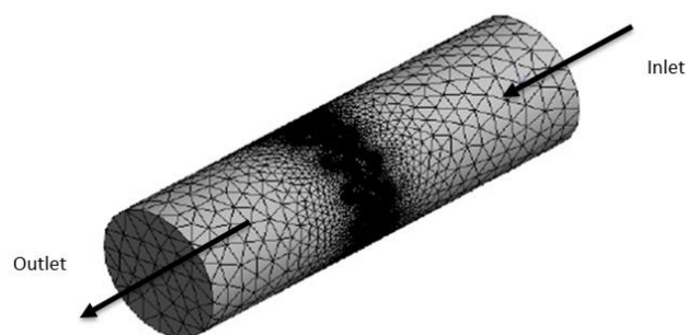
Fig. 2. Tetrahedral mesh of the computational domain
