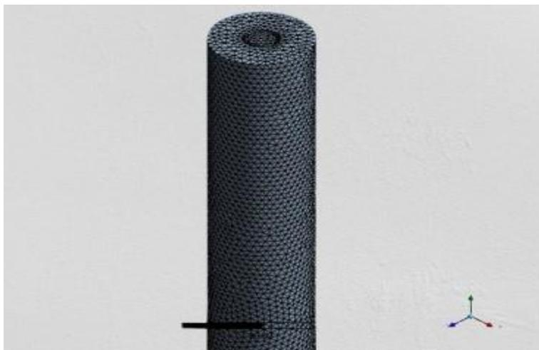
**Fig. 3.** The result of the generated of mesh PU spray nozzle model
