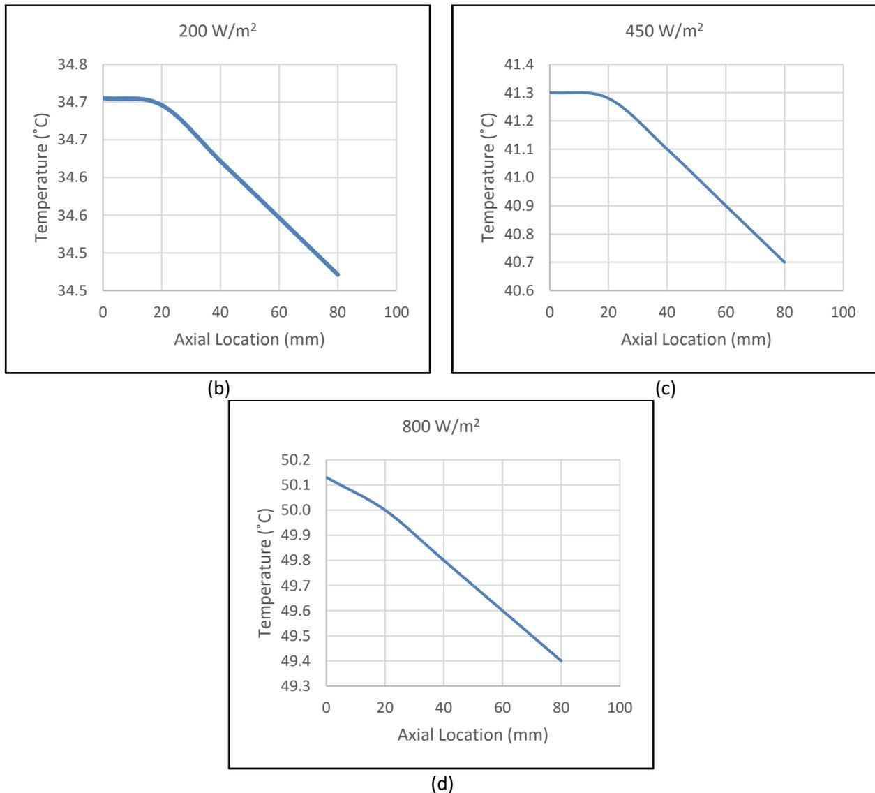
**Fig. 7.** (a) Axial Temperature Distribution (b) Axial Temperature Profile at 200 W/m<sup>2</sup> (c) Axial Temperature Profile at 450 W/m<sup>2</sup> (d) Axial Temperature Profile at 800 W/m<sup>2</sup>
