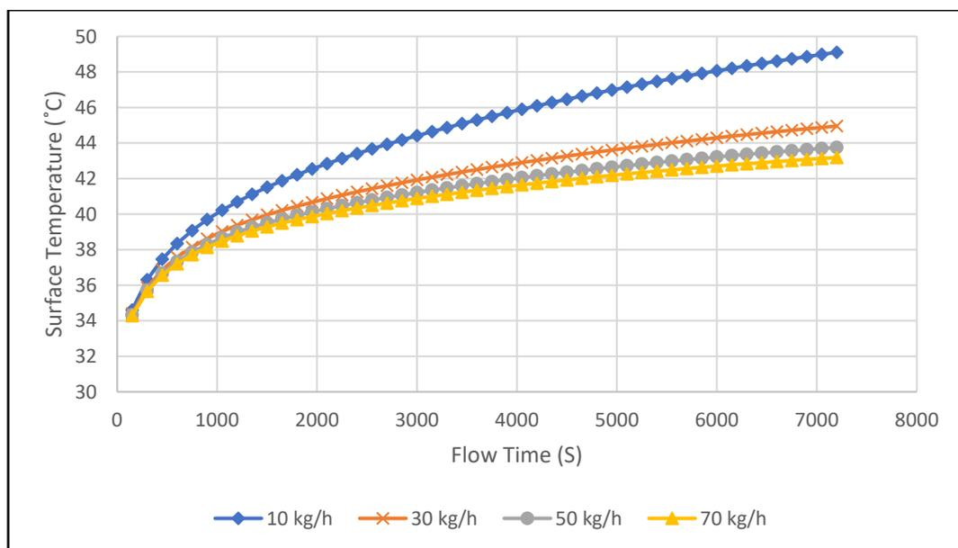
**Fig. 3.** Surface Temperature of PVT-PCM on Various Mass Flow Rate at Constant Solar Irradiance 450 W/m<sup>2</sup>
