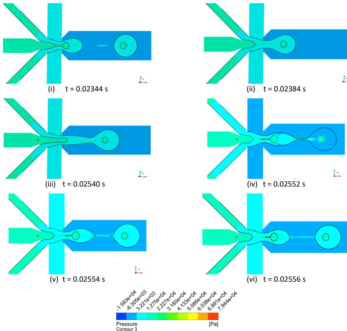
**Fig. 7.** Pressure contour on droplets evolution at the junction
