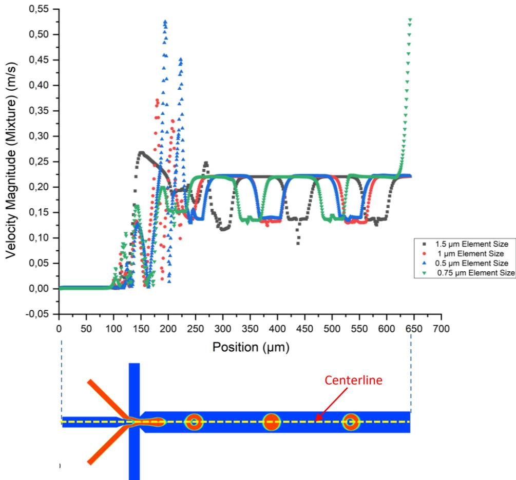
**Fig. 3.** Mesh independency analysis with the use of velocity magnitude profile along centerline vs. position along the x-axis
