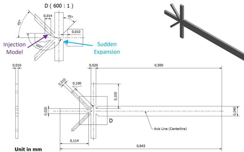
**Fig. 1.** The modified flow focusing device
