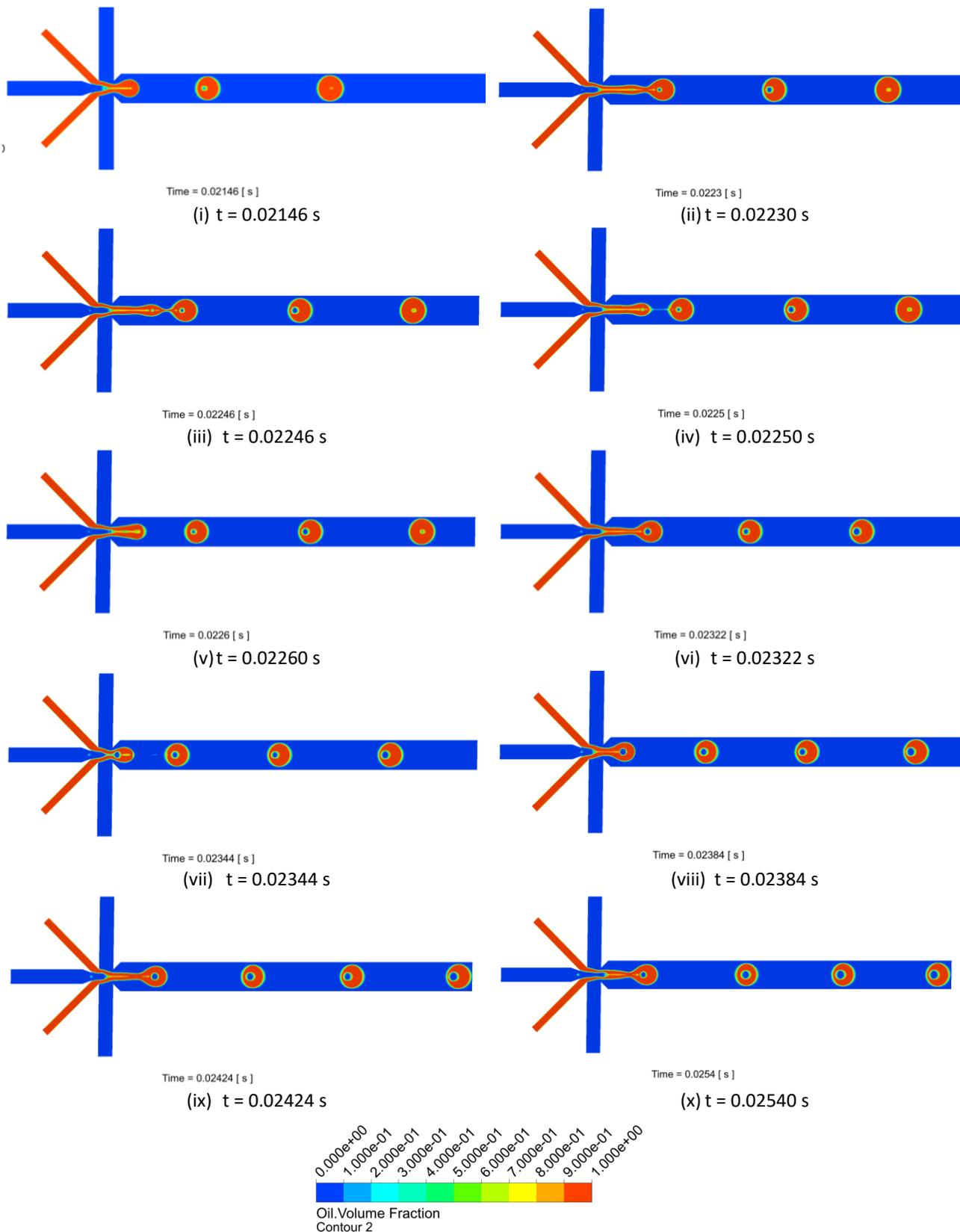
**Fig. 6.** Droplets evolution based on olive oil volume fraction
