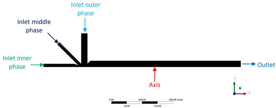
**Fig. 2.** Scheme of boundary conditions in the pre-CFD process
