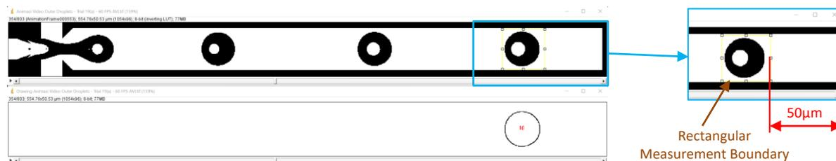
Fig. 4. Outer droplets diameter estimation
