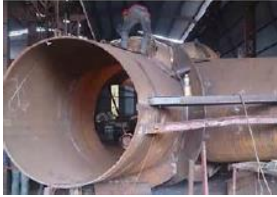
Fig. 3. Branch pipe t-joint with central reinforcement [8]
