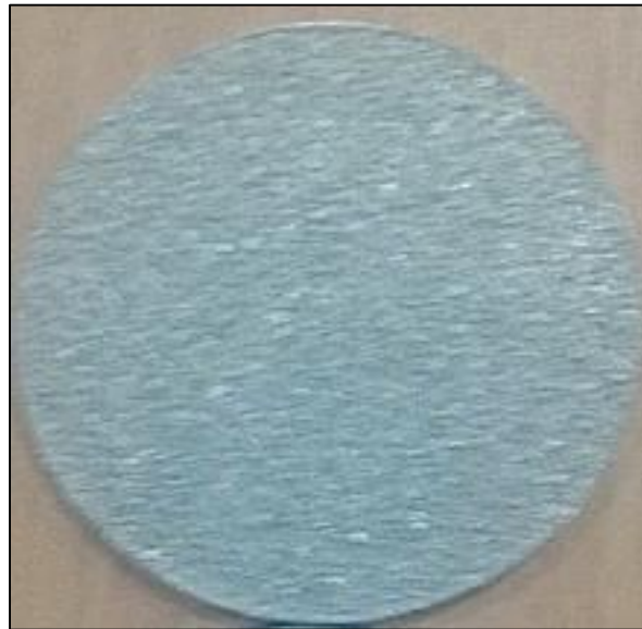
Fig. 1. Sintered stainless steel Porous Media R200
