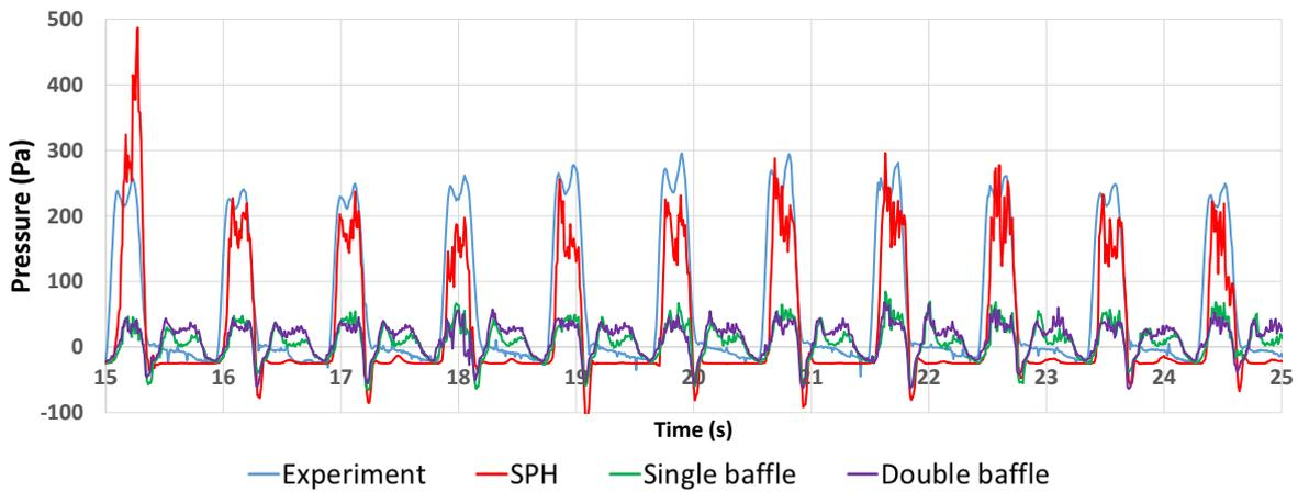
Fig. 7. Comparison of dynamic pressure without and with baffles
