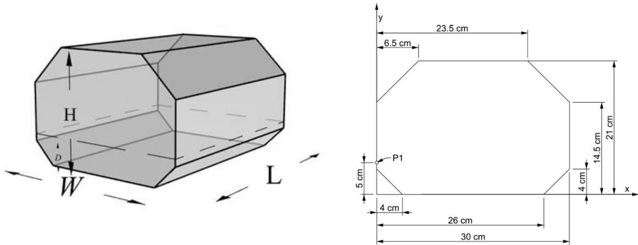
Fig. 2. Sketch of numerical domain and position of pressure sensor
