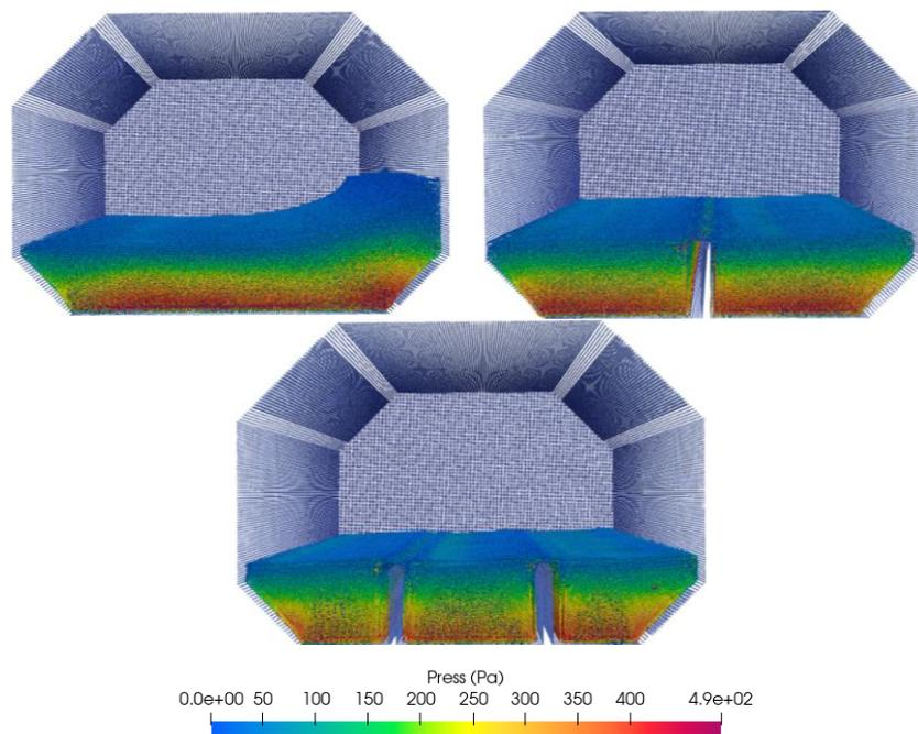
Fig. 8. Snapshot of dynamic pressure for sloshing without and with baffles with  $t = 15.20$  s
