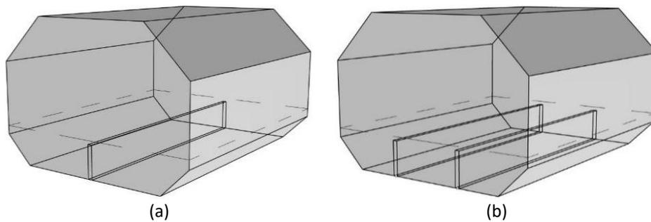
**Fig. 5.** Sketch of the prismatic tank with a (a) single-vertical baffle, and (b) double-vertical baffle
