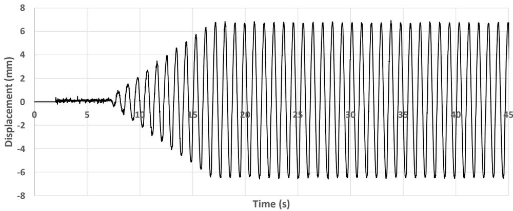
Fig. 3. The time history of tank displacement in sway motion
