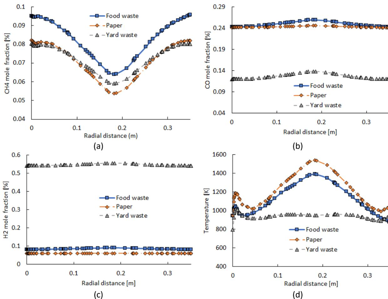
**Fig. 3.** Comparison of syngas composition between food waste, paper and yard waste in oxidation zone for the component of (a) CH<sub>4</sub>, (b) CO, (c) H<sub>2</sub>, and (d) temperature
