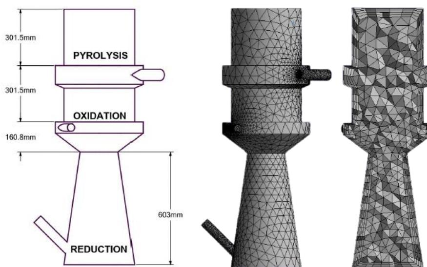
**Fig. 1.** Gasification zone and structure tetrahedron mesh
