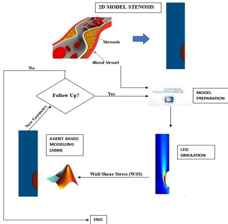
**Fig. 4.** Couple computational framework. Combining computational fluid dynamics (CFD) simulation using COMSOL Multiphysics and agent-based modelling (ABM) simulation using MATLAB to examine the development of stenosis in blood flow
