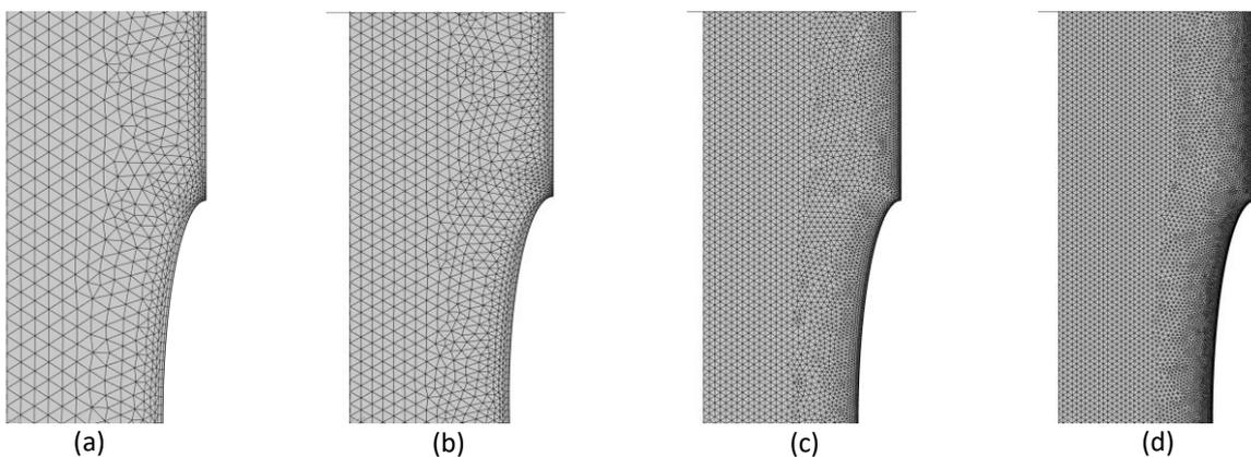
**Fig. 3.** Mesh with various element sizes with partially magnified section. (a) Mesh 1, normal element size (b) Mesh 2, fine element size (c) Mesh 3 with a finer element size (d) Mesh 4, extra fine element size
