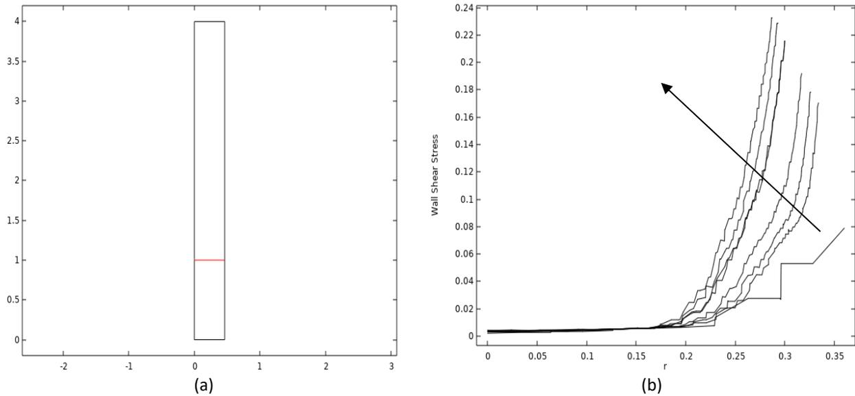
Fig. 9. Wall shear stress (b) at the line cut (a) for the various progression of the stenosis
