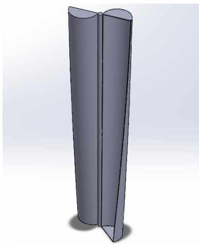
Fig. 1. Design of Savonius wind turbine model
