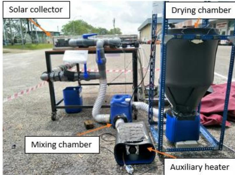
**Fig. 6.** Setup for a solar drying system
