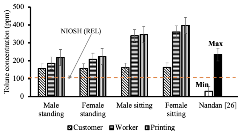
Fig. 6. Bar chart of toluene concentration during Case 3
