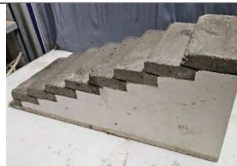
(8) Setup the RCC layers in Mold
