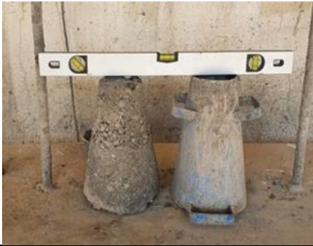
(3) Test the zero-slump requirement
