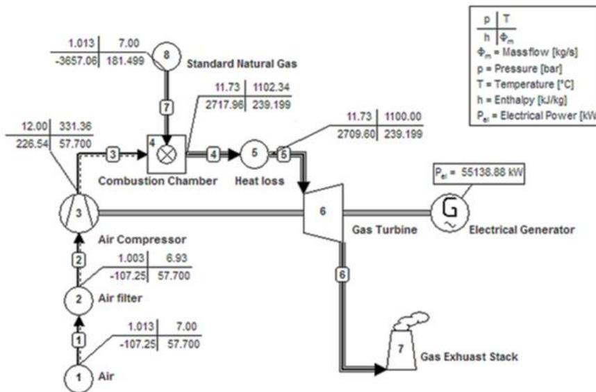
Fig. 2. Sketch diagram of a single shaft (GTPP)
