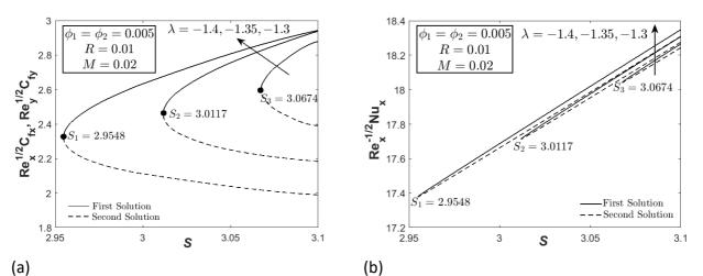
**Fig. 2.** (a) Skin friction coefficients, and (b) thermal rate of Fe<sub>3</sub>O<sub>4</sub>-CoFe<sub>2</sub>O<sub>4</sub>/water towards suction with variation of shrinking parameter
