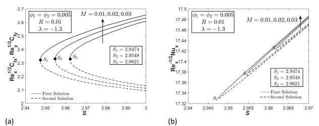
**Fig. 3.** (a) Skin friction coefficients, and (b) thermal rate of Fe<sub>3</sub>O<sub>4</sub>-CoFe<sub>2</sub>O<sub>4</sub>/water towards suction with variation of magnetic strength
