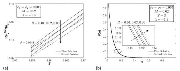
Fig. 4. (a) Thermal rate, and (b) temperature profile of  $Fe_3O_4$ -CoFe<sub>2</sub>O<sub>4</sub>/water with variation of radiation parameter
