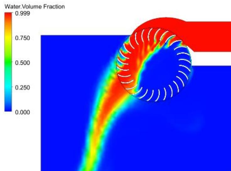
Fig. 6. Water volume fraction contour in the turbine symmetry plane
