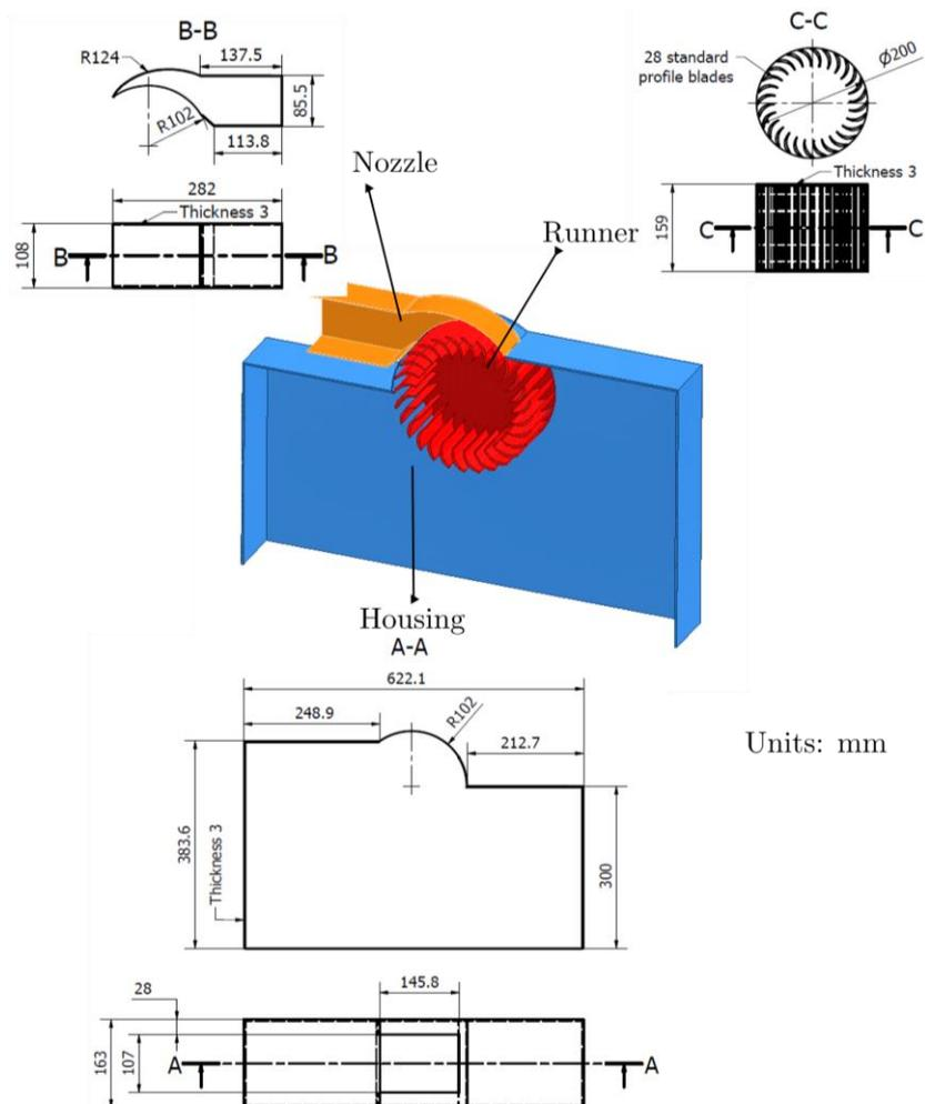
**Fig. 2.** Isometric view of the CAD model of the designed MBT, with the structural dimensions of each element
