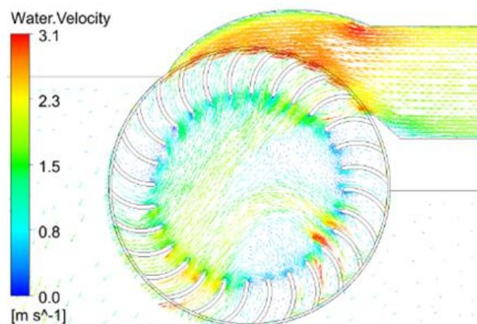
Fig. 8. Velocity vectors in the symmetry plane of the MBT
