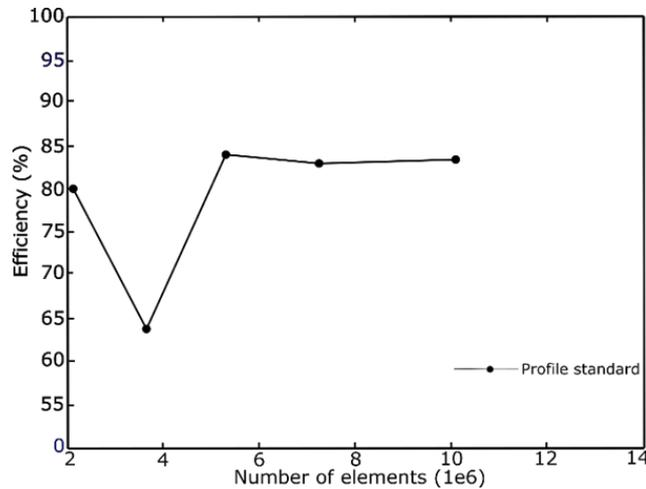
Fig. 5. Mesh independence for the model under study
