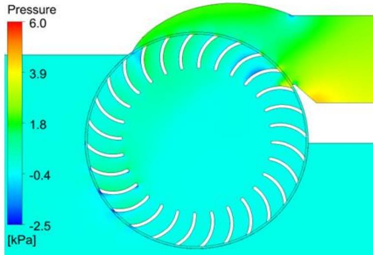
Fig. 7. Total pressure contour in the symmetry plane of the MBT
