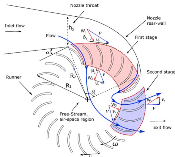
**Fig. 1.** Geometrical scheme of the MBT and the particle in motion within the rotating reference frame. Source: Adapted from [9]
