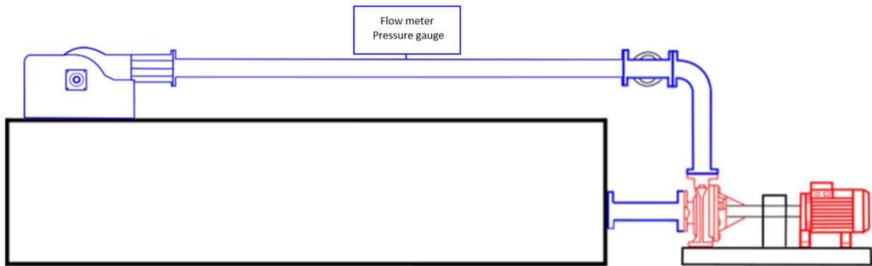
**Fig. 3.** Diagram of the hydraulic bench
