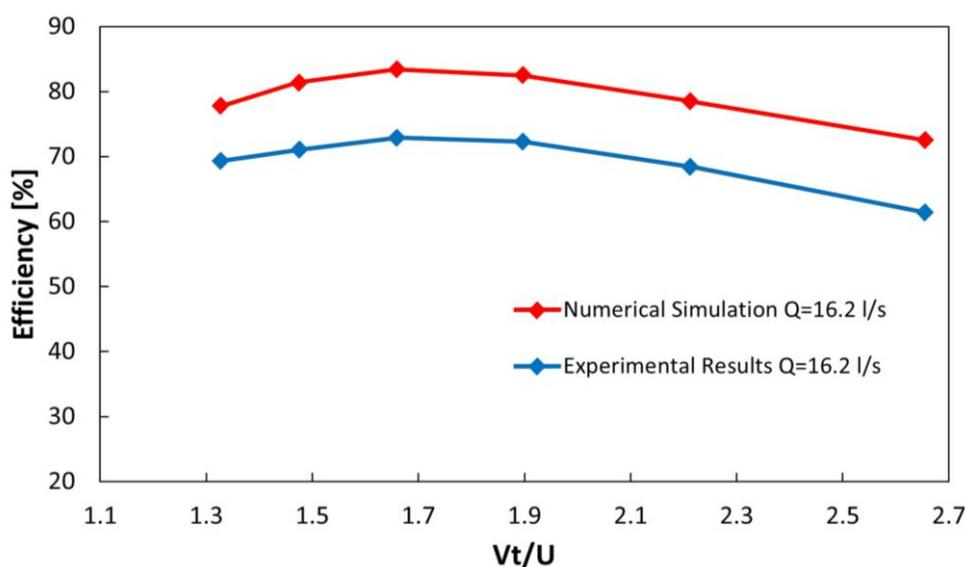
Fig. 10. Experimental and numerical curves of efficiency vs. speed for different flow conditions
