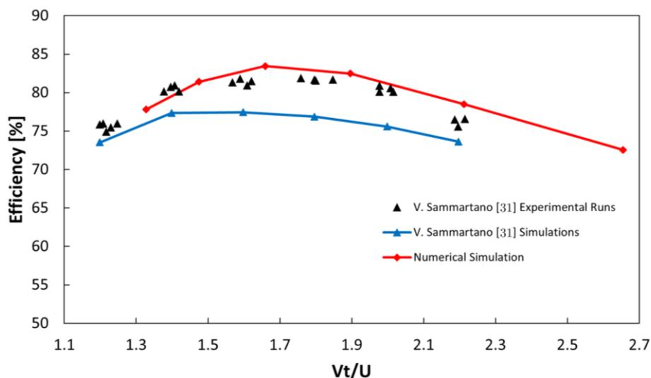
**Fig. 9.** Efficiency of MBT as a function of the speed ratio obtained for the present study and by the research by V. Sammartano [31]
