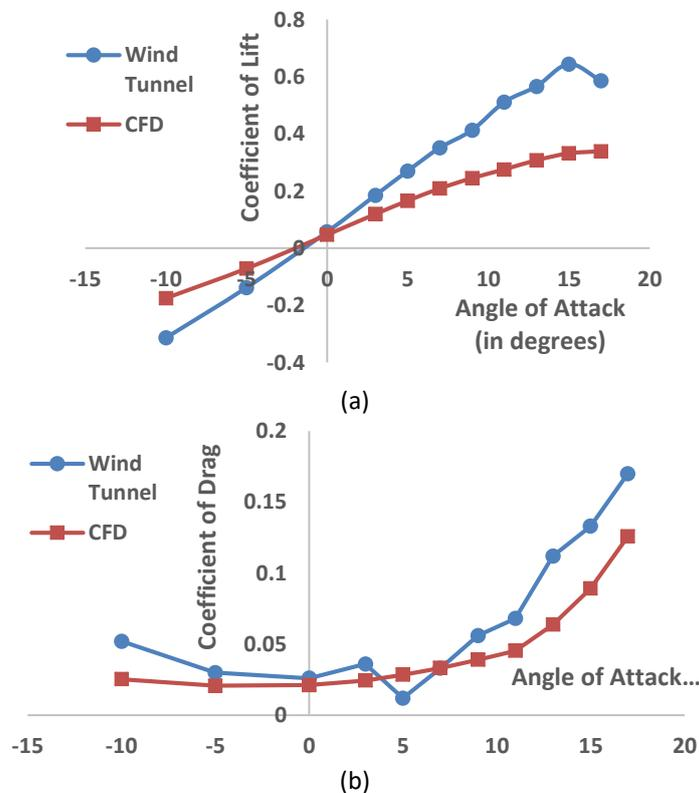
**Fig. 4.** Comparison of lift and drag coefficients from CFD simulation and reference wind tunnel test (a) Lift coefficient (b) Drag coefficient
