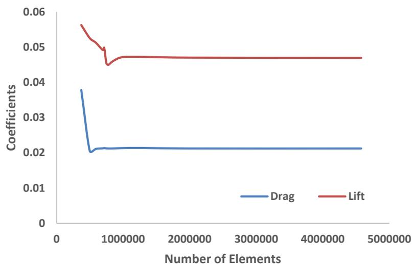
Fig. 5. Mesh convergence study for the CFD simulation analysis
