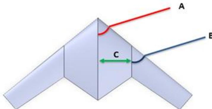
**Fig. 2.** Design variables for the parametric study: A (inboard sweep angle), B (outboard sweep angle), C (inboard wing span)
