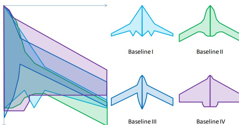
**Fig. 1.** Examples of BWB UAV designs by FTTC [11]
