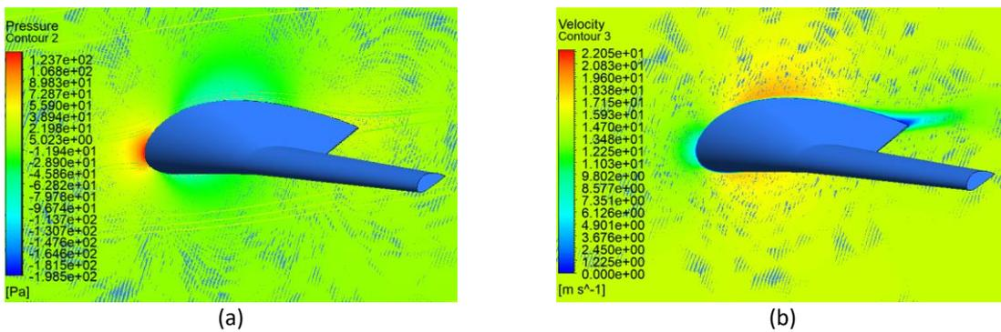
**Fig. 3.** CFD simulation results for current Baseline-VII design (a) Pressure contour (b) Velocity contour
