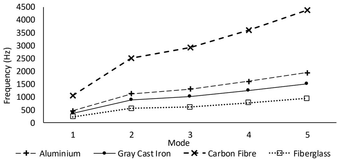
Fig. 5. Natural Frequency for Intake Manifold
