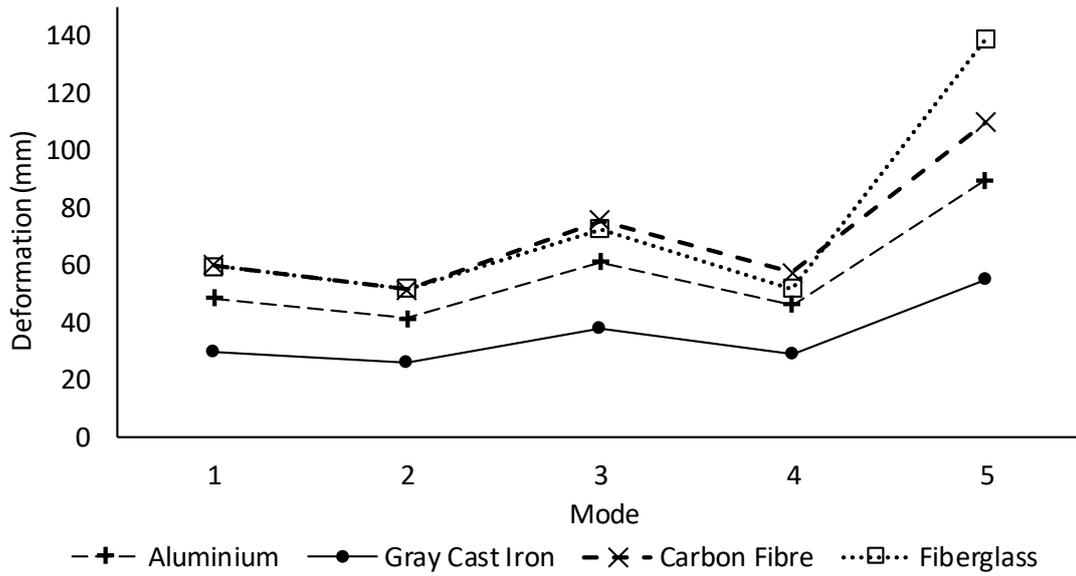
Fig. 4. Maximum deformation for intake manifold
