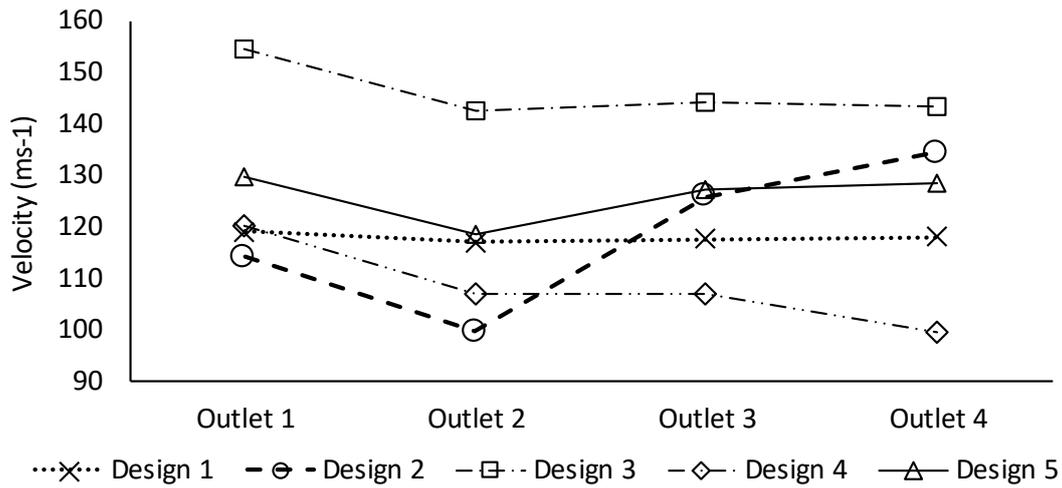
**Fig. 2.** Average Velocity for Each Design in Each Outlet
