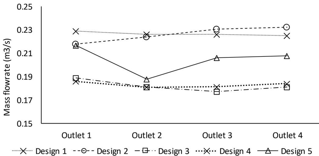
**Fig. 3.** Mass Flowrate for Each Design in Each Outlet
