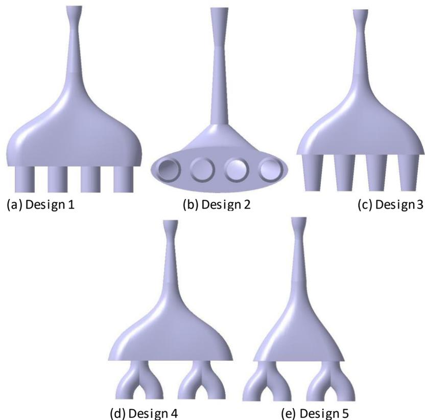
**Fig. 1.** Intake manifold designs
