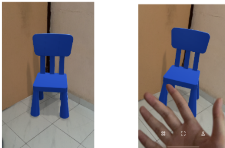
Fig. 3. Object rendering and occlusion test on device with LiDAR
