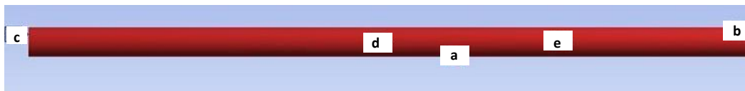
Fig. 6. Boundary condition in the model geometry (a) Pipe wall (b) Outlet (c) Inlet (d) Leak outlet 1 (e) Leak outlet 2
