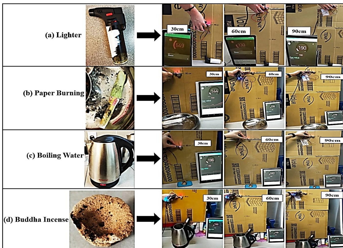
Fig. 15. Gas detection at different sensor placement distances
