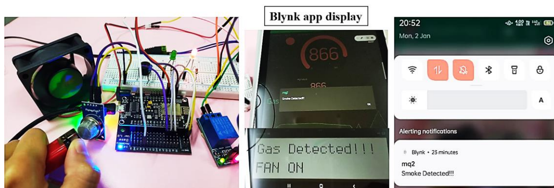
Fig. 13. Gas-detected condition circuit setup, Blynk display, and pop-up alert notification
